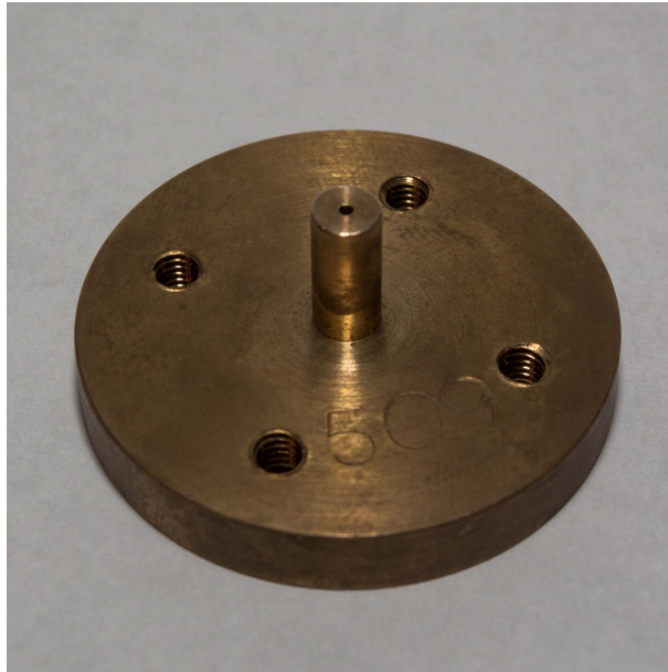
Figure 1.3: Photograph of brass gas jet with 1 mm diameter gas outlet.
