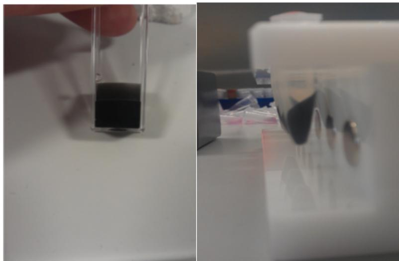
**Figure 4.2 – (Left) Photograph of unshelled magnetite nanoparticles. (Right) Photograph of magnetite nanoparticles on a magnetic separation rack, illustrating the magnetic nature of the nanoparticles.**
