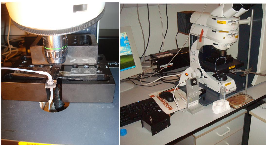
**Figure 3.31** –Photographs of flow cell construction. The micro-cuvette flow cell is positioned with the optical window directly below the microscope objective, and the inlet of the cell is attached to tubing from a peristaltic pump for sample delivery and removal. The magnet is positioned introduced through the void in the microscope stage, directly beneath the flow cell.
