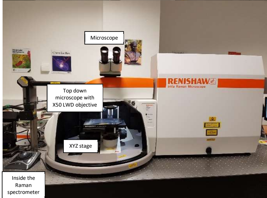
Figure 21: Photographs with labels of the Renishaw InVia Raman microscope fitted with 532 and 633 nm lasers
