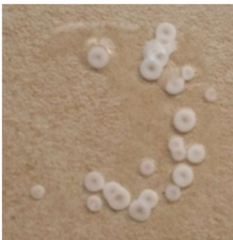
Figure 3: Photograph showing crystallised glucose on a lino section of dimensions shown in Figure 1H.
