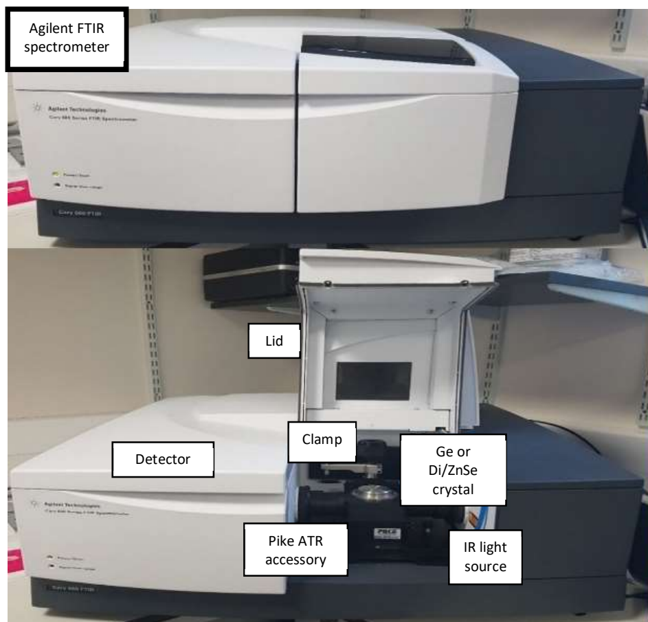
Figure 17: Photographs with labelling for the Agilent Cary 660 benchtop spectrometer and Pike ATR accessory
