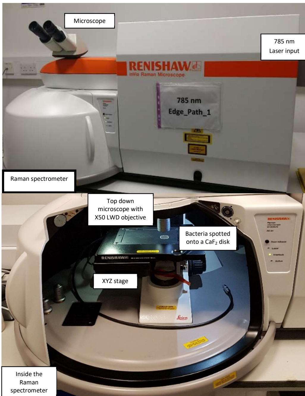
Figure 22: Photographs with labels of the Renishaw InVia Raman microscope fitted with a 785 nm laser
