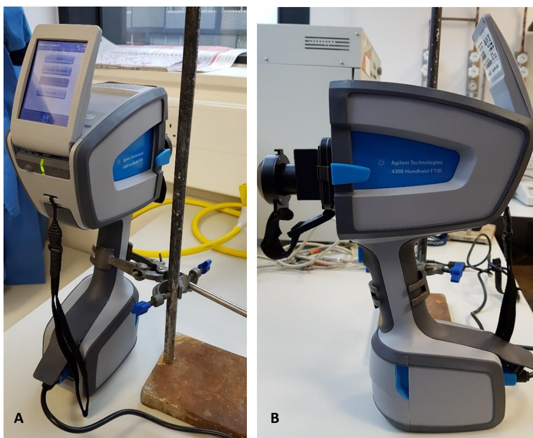
Figure 1: Figure showing the handheld spectrometer setup using a clamp to hold the spectrometer in place and the PDA raised for ease of use (A) along with a side view showing the attachment of the diffuse reflectance accessory with a coarse Gold reflectance cap fitted (B).
