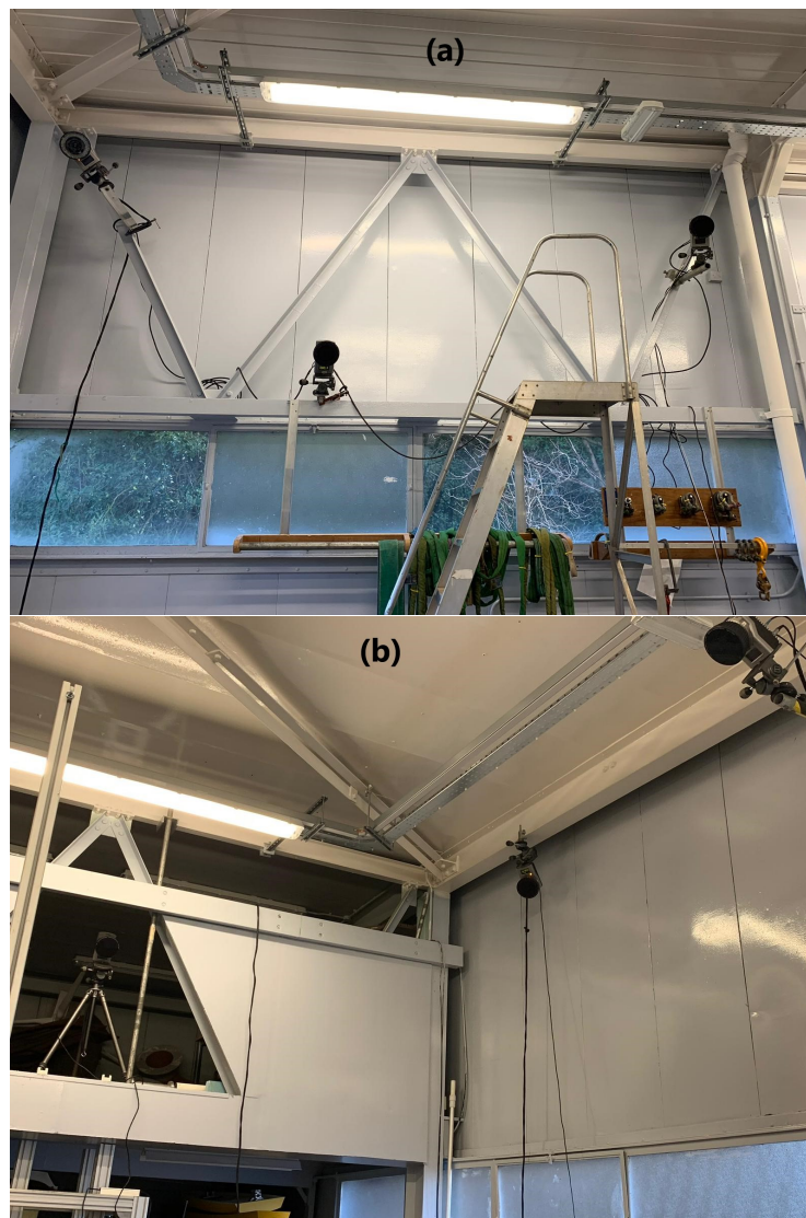
Figure 3.2: Schematic of the in-air experimental set-up with (a-b) qualisys camera above.
