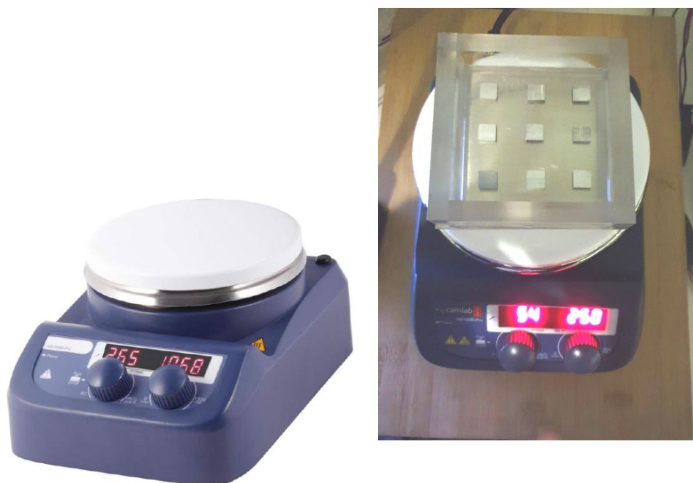
Figure 78: MS-H280-Pro Round ceramic coated Steel Hotplate.
