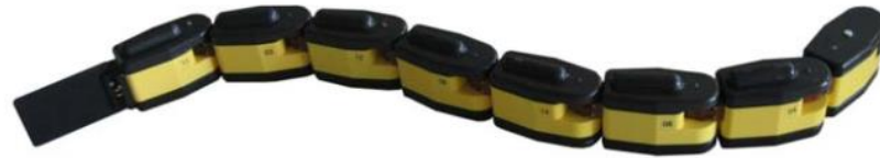
(a) A serial-like Multi-Body model: Amphibot III (Porez et al., 2014b)
