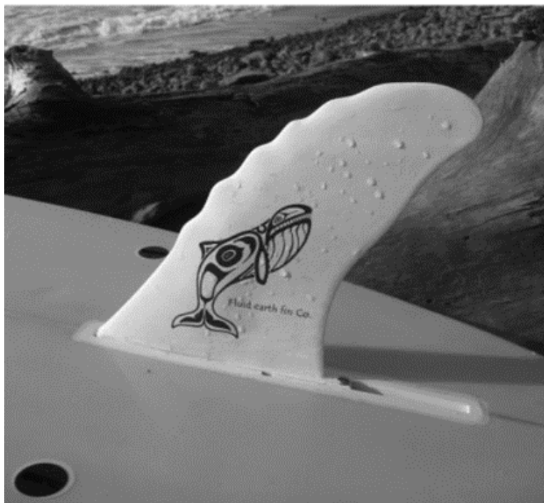
Figure 2.25: LE tubercles applied to the fin of surfboard courtesy of H.Swales and Fluid Earth [82]
