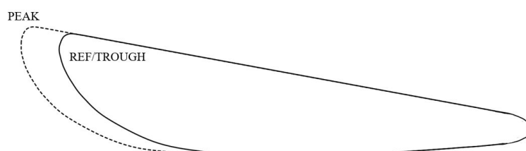
Figure 3.3: Cross-section tubercle peak and trough profiles
