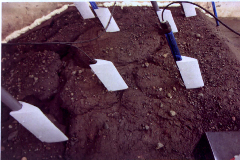
Figure 8.16 Eroded slope and the half crest.
