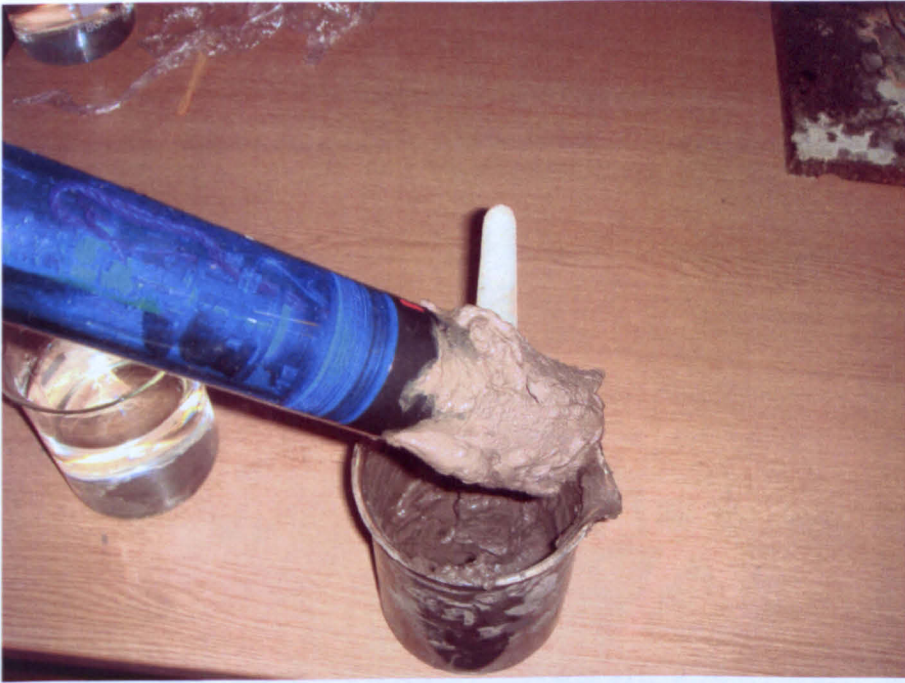
Figure 5.20 Ceramic cup covered with the slurry paste.
