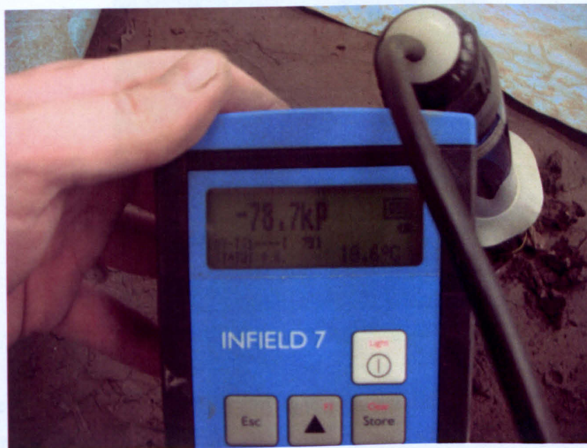
Figure 5.25 UMS INFIELD 7b Pressure Reading Unit used for controlling insertion pressure.
