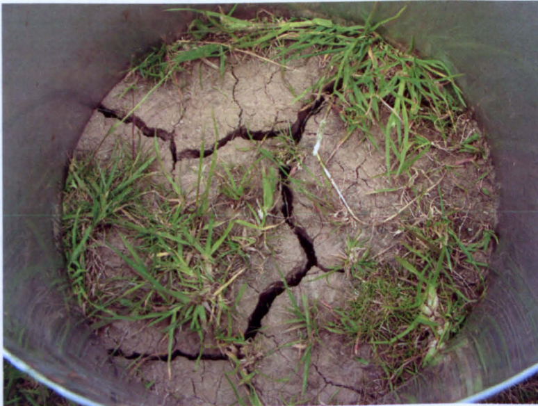
Figure 3.19 Surface crack pattern within the inner ring.
