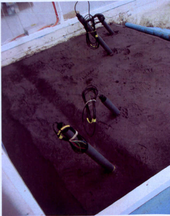
Figure 5.18 TDR probes installed on the crest.
