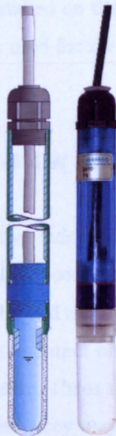
Figure 5.6 Soil water tensiometer sensor - T4e (after UMS).
