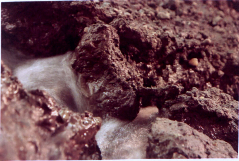
Figure 8.24 Visible small collapse in the clay block.
