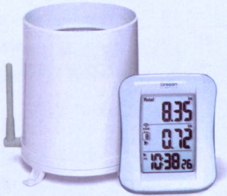
Figure 5.9 Oregon Scientific Wireless Rain Gauge with self-emptying rain cup and the indoor gauge module.
