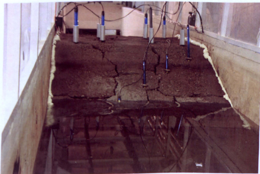
Figure 8.5 Channel filled with water to the level of the first tensiometer.
