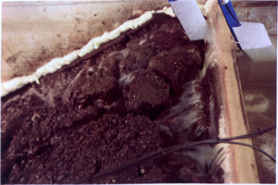
Figure 8.22 Collapsing clay block.
