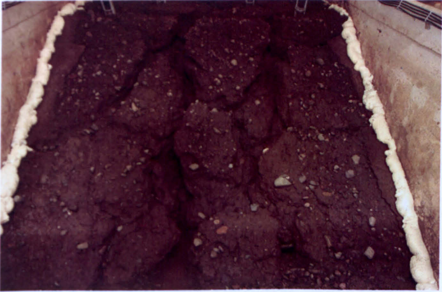
Figure 8.18 Eroded slope with the two flow paths visible in the middle of the slope.
