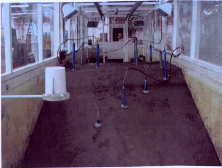
Figure 4.28 Environmental chamber with embankment and installed sensors.
