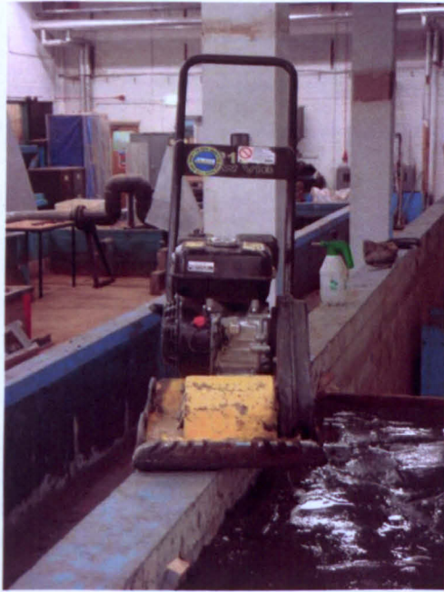
Figure 4.20 85 kg vibrating plate used for compaction.
