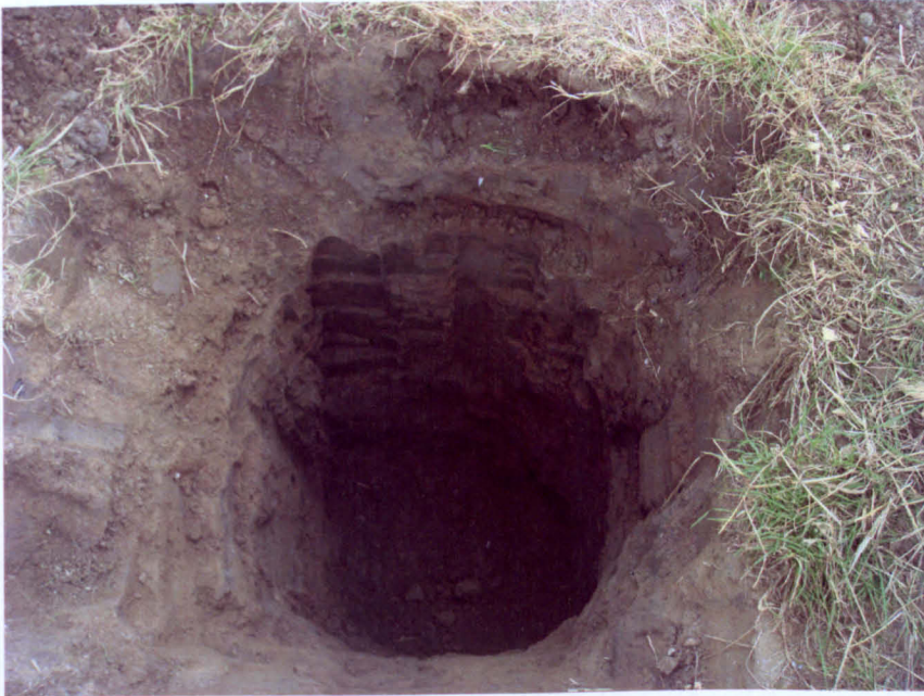
Figure 3.38 Trial trench excavated at Lancaster embankment.
