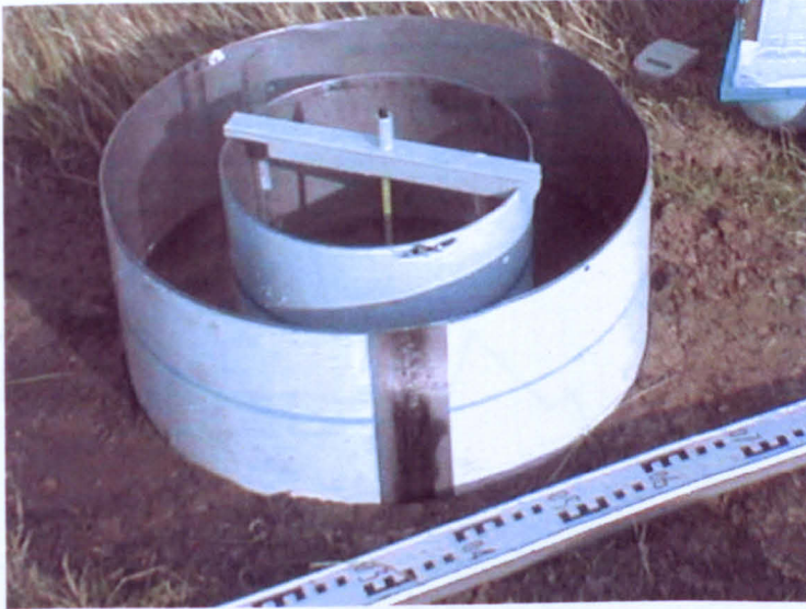
Figure 3.16 Double ring infiltrometer apparatus.
