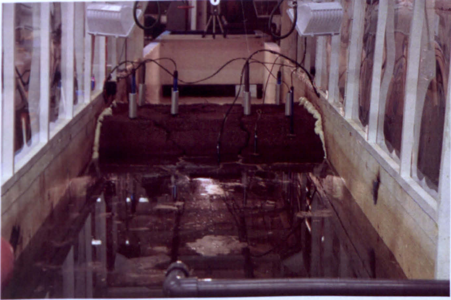
Figure 8.7 Upstream side of the embankment with the water level 20 cm below the crest.
