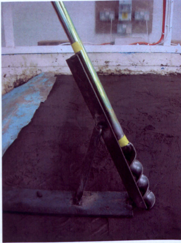
Figure 5.15 Supporting steel angle with the auger.
