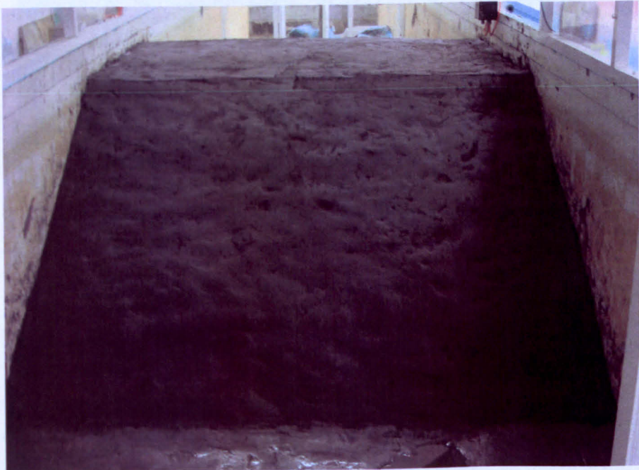
Figure 4.27 Final shape of the embankment.
