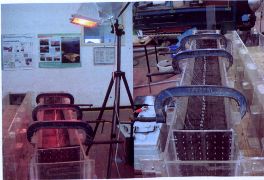
Figure 6.2 Experimental setup with infra-red heater and electrodes installed.
