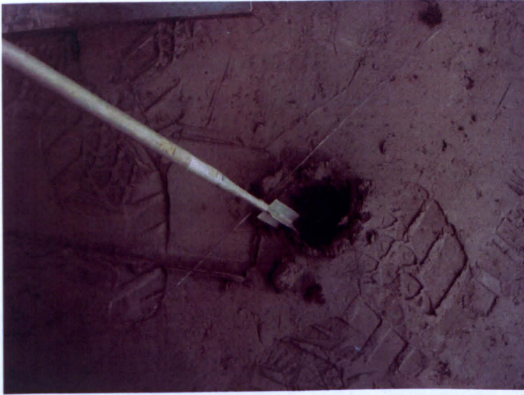
Figure 5.17 Field inspection vane tester for undrained shear strength measurements.
