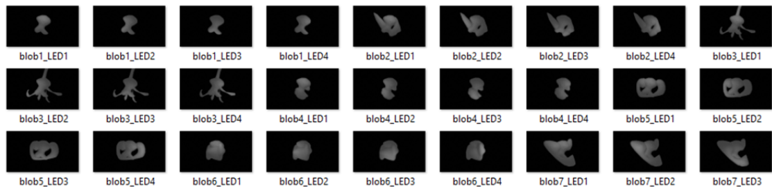
Figure 7.10: Selection of rendered images using the Blender script. Four images are rendered for each blobby shape, one image for each illumination direction.
