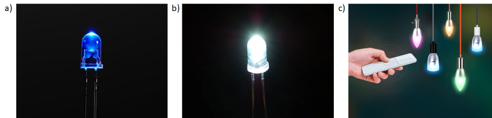
Figure 2.1: a) Blue LED, b) White LED and c) smart-lighting using LED bulbs.
