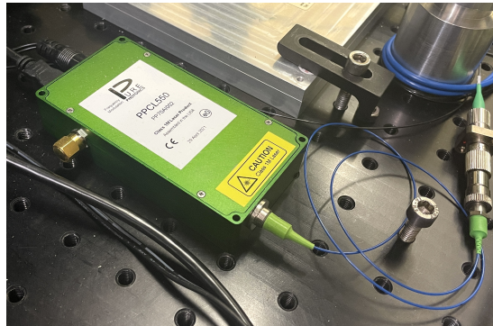
Figure 4.5: Pure Photonics PPCL550 tuneable telecoms laser with fiber output. The laser package is very compact, with a length of less than 10 cm.
