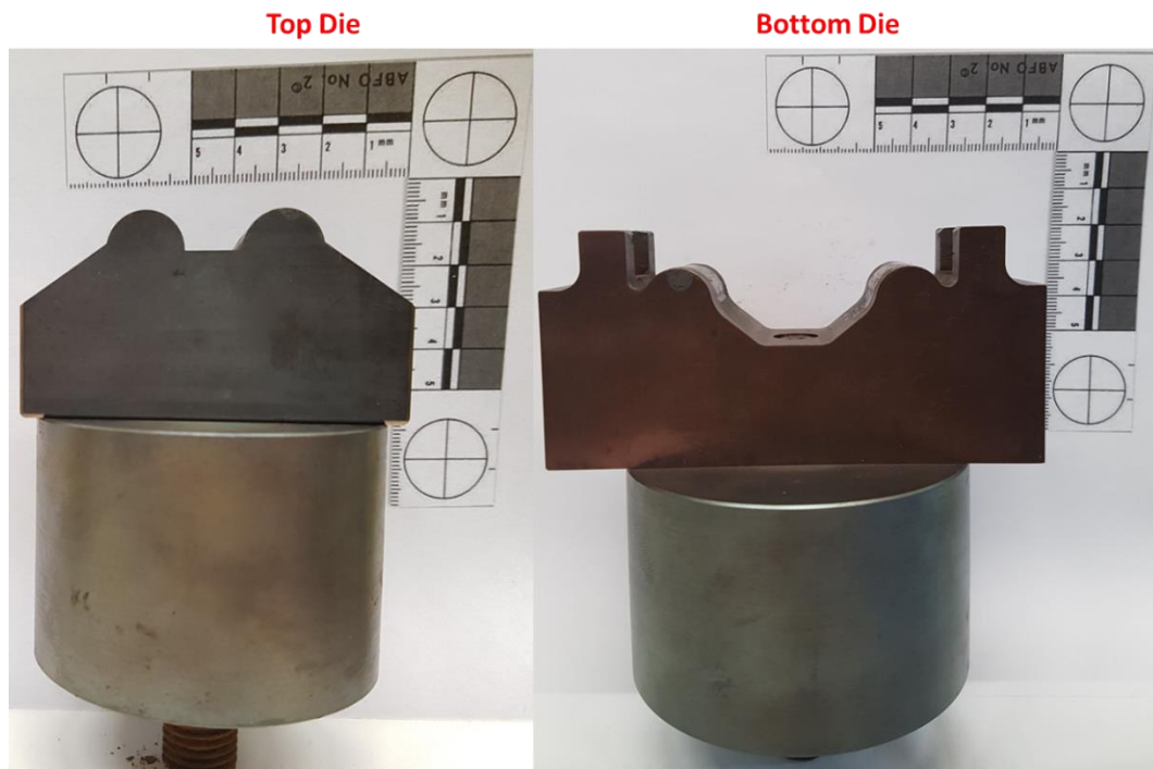
Figure 4.7: Second design iteration of the four-point bending die
