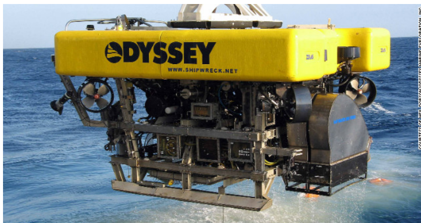
Figure 2: 8 Ton ROV used for marine salvage [87]
