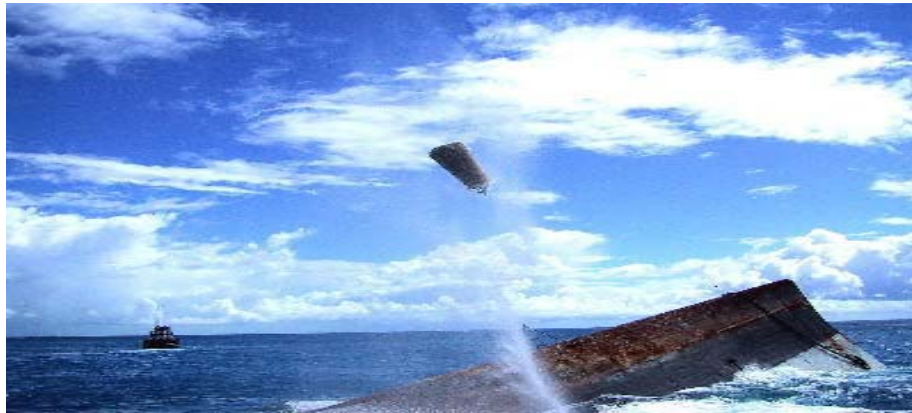
Figure 5: A 25 ton capacity lift bag that broke free from USS Spiegel Grove during the salvage operation. The lift bag reached an altitude of approximately 30 meters. Photo - courtesy of
