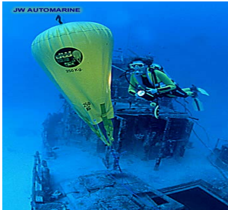
Figure 3: Scuba diver attaching inflated bags to the sunken vessel. Photo - courtesy of J W Automarine [32, 61]
