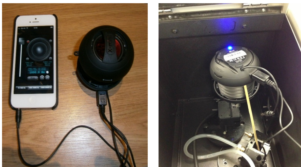
Figure 31 Experimental set-up, showing the speaker connected with an iphone 5 and inside the fluorimeter (2 cm above the fluorescence cuvette) to provide liquid vibrations.
