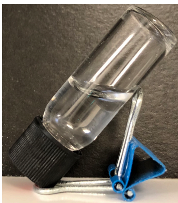
Figure 4.37 Picture of Fmoc G after 6 days. 10 mM of Fmoc G was added to 1 mL of 100 mM, pH 8 phosphate buffer.
