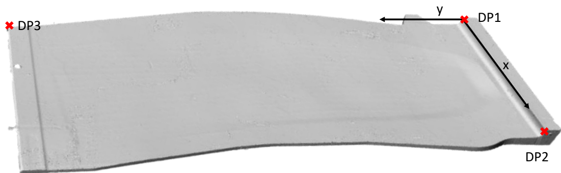
Figure 3.2.26: Datum points chosen on part to establish scan reference axes.
