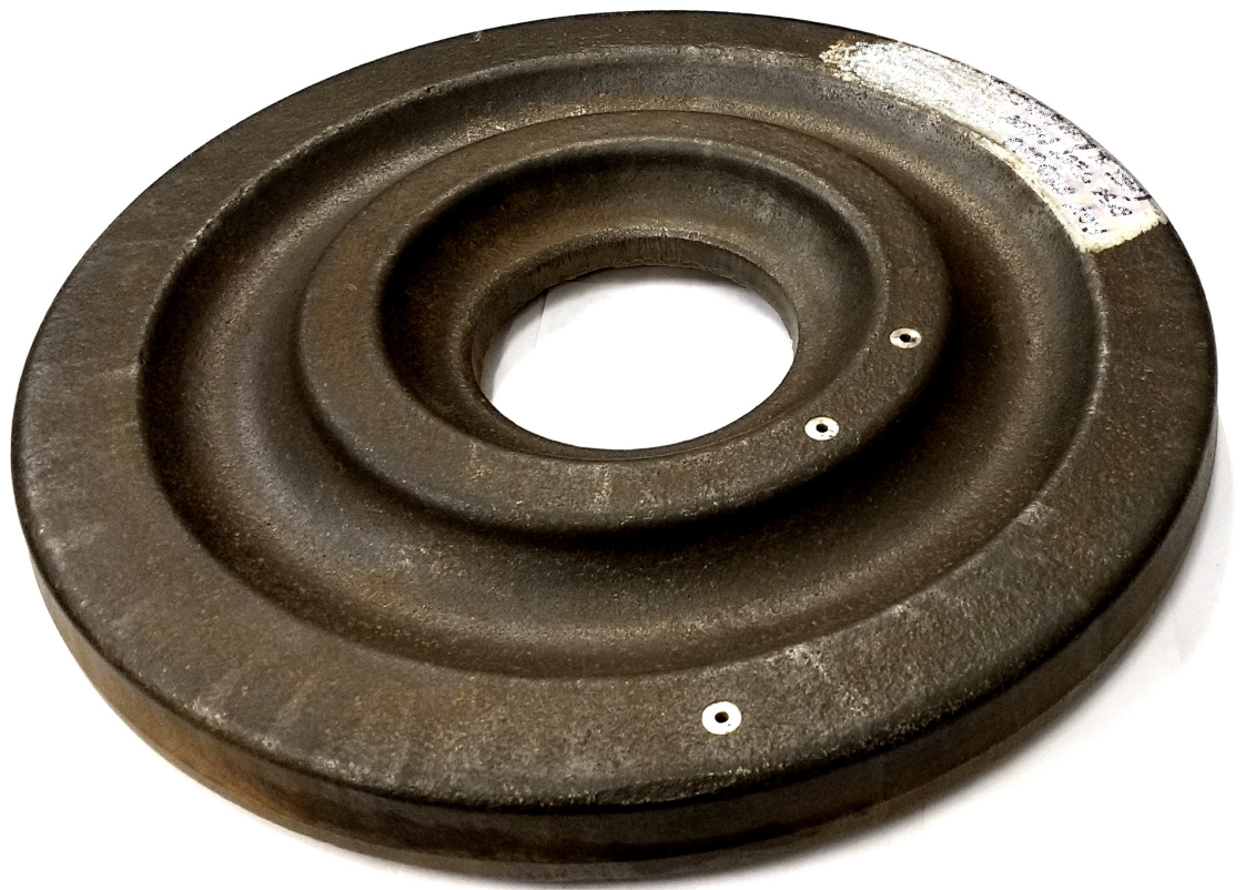
Figure 5.2.3: Photograph of black forged disc. Diameter is roughly 300 mm.
