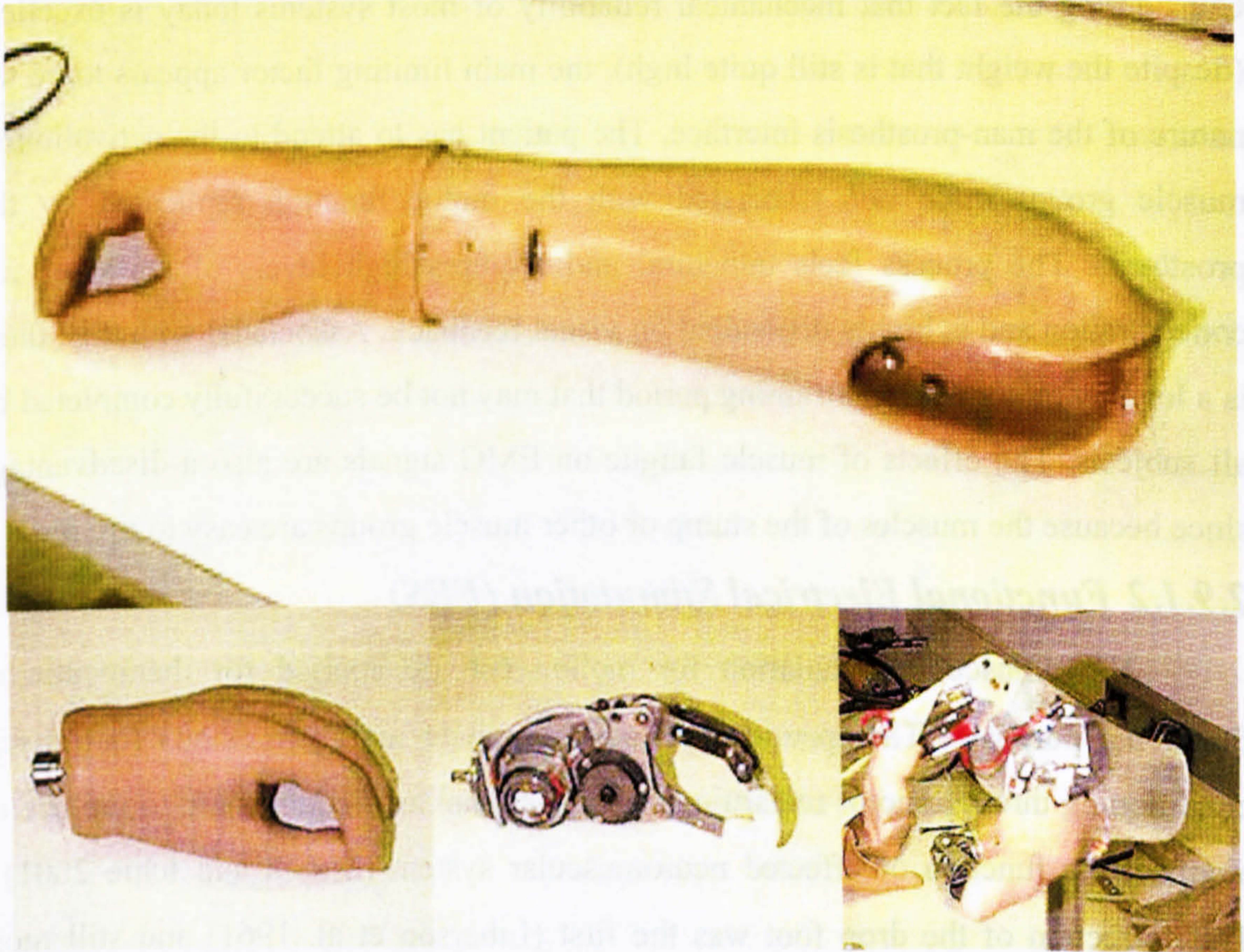
Fig. 2.30 Typical below elbow myoelectric prosthesis. Small electrodes that fit intimately against the skin detect the minute residual muscle electrical activity as it contracts. When one is detected, circuitry tells the motor to open or close. The inner workings of the myoelectric arm reveal the circuit board, electrical connections, and electric motor. Adapted from Northwestern University Prosthetics and Orthotics Centre Website http://www.nupoc.northwestern.edu 2004.
