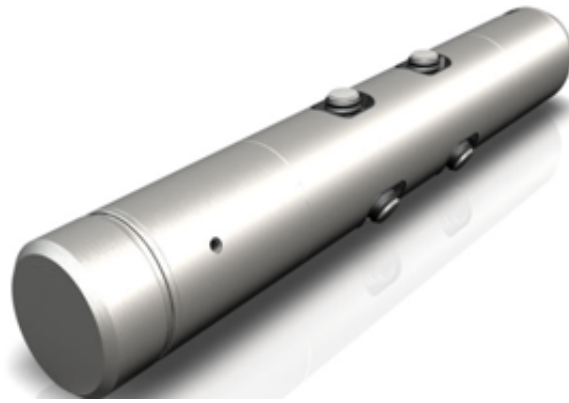
Figure 3.15: The trepanning tool, which can cut small cylindrical samples of irradiated graphite from fuel channels, for testing. Diagram courtesy of EDF Energy.
