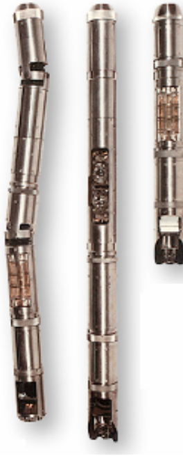
Figure 3.13: The articulated camera which can be inserted to visually inspect fuel channels. Diagram courtesy of EDF Energy.
