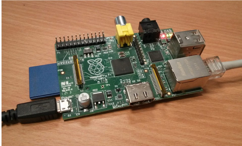
Figure 8.36: A Raspberry Pi computer. For testing, a JADE platform is created on the device running in a Linux based OS which boots straight from an SD card.
