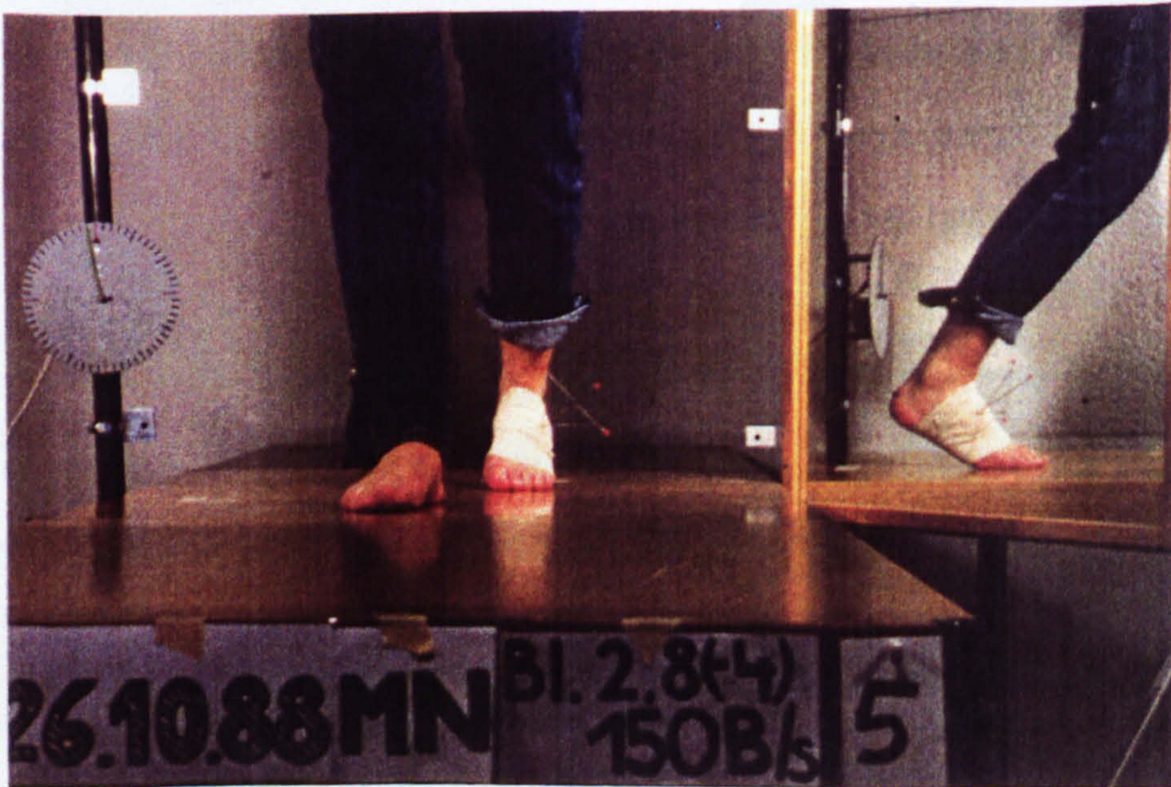
Figure 5-3 b View through camera lens showing marker triad on foot and stationary reference points on split picture
