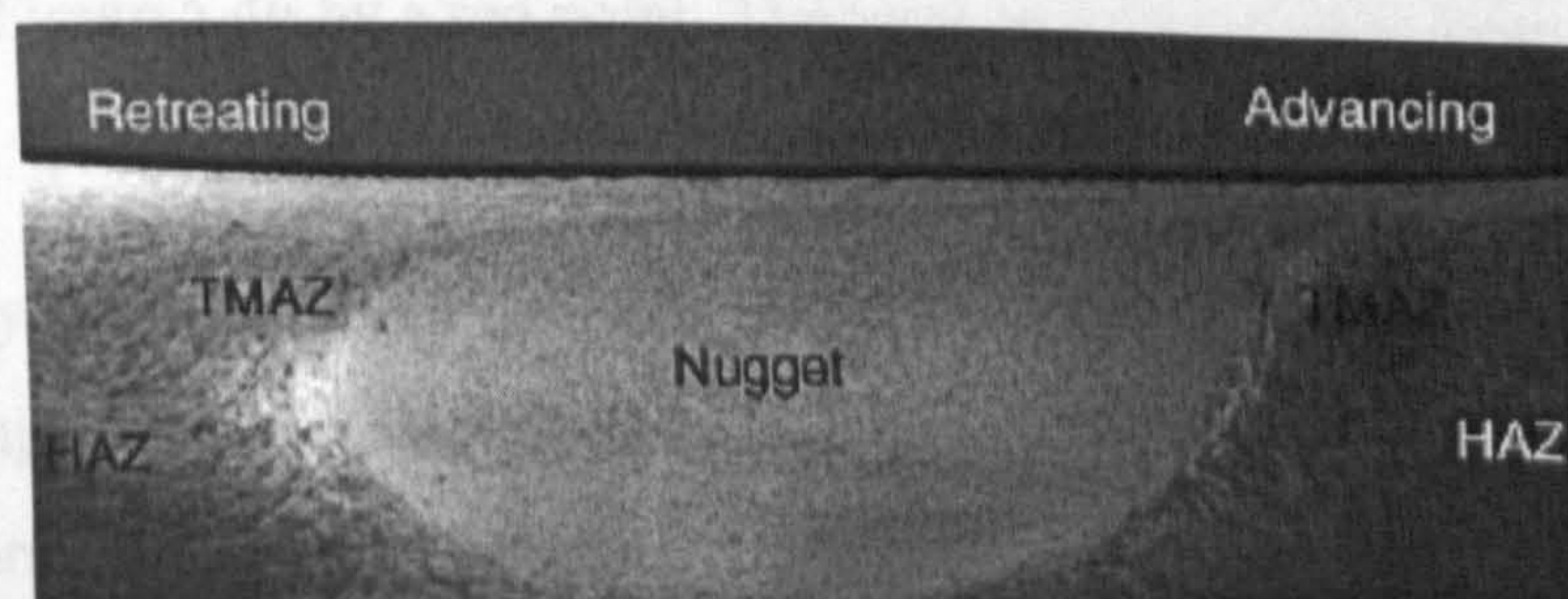
Figure 5.44 Microstructure classification of friction stir welds [5.25].
