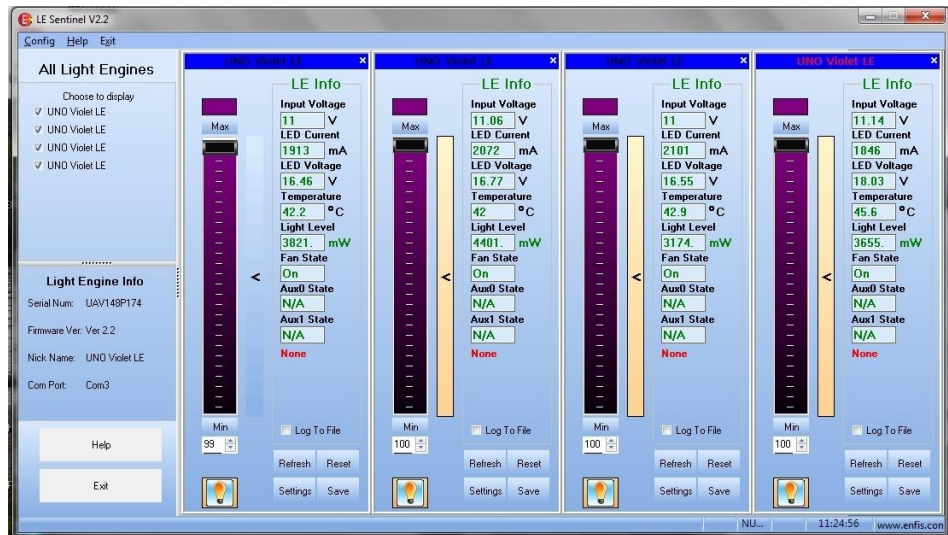
Fig. 9.8. Display of the LE sentinel (V2.2) software on a computer screen. This software is supplied by ENFIS Ltd., UK, for controlling and monitoring the 405 nm LED light engines.
