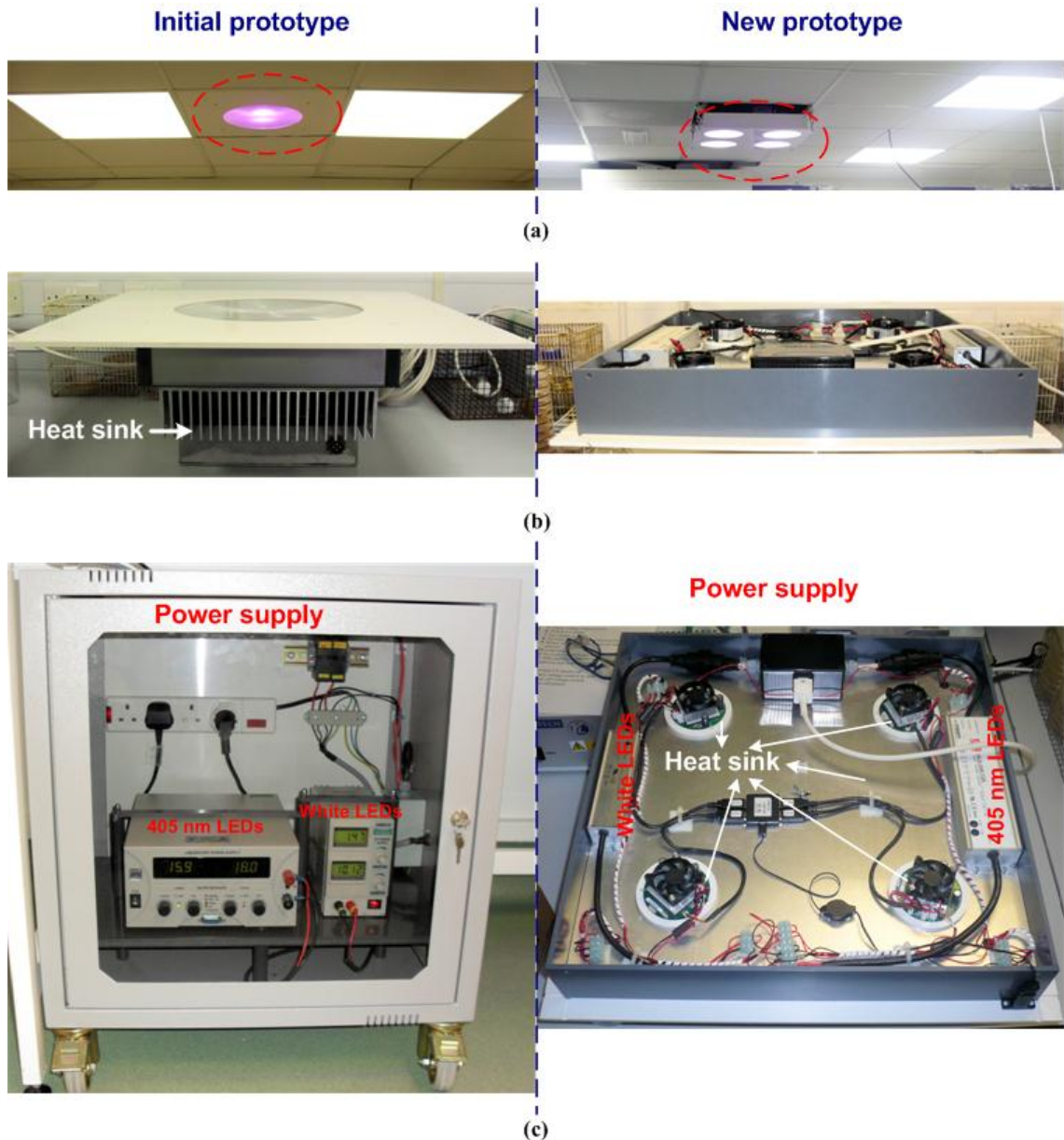
Fig. 9.18. Comparative design of aspects of the initial prototype and the new prototype HNS-light EDS: a) light emitted from initial prototype still produced dominant violet illumination whilst the new prototype emits light close in appearance to laboratory lighting. b) dimensional comparison between the initial prototype and the new prototype, and c) power supply to drive the EDS: detached and bulky for the initial prototype whilst small and integrated into the system for the new prototype.
