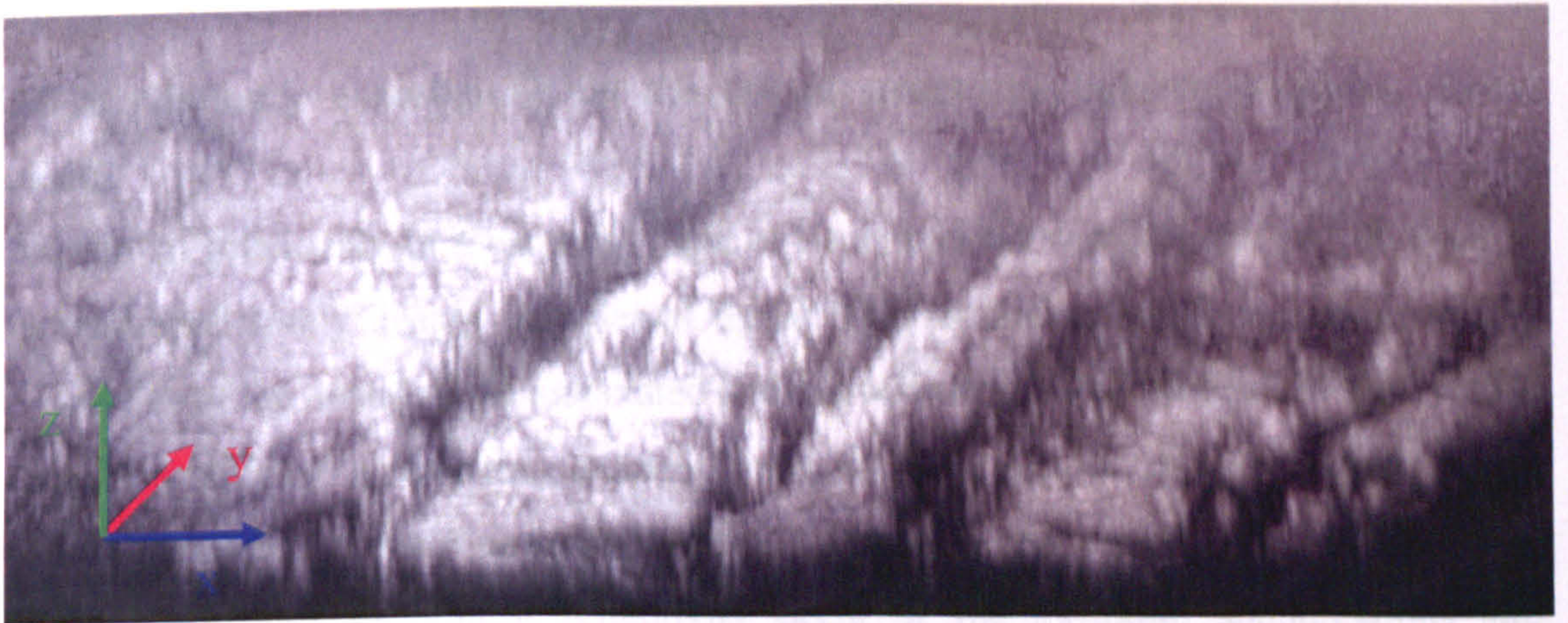
Figure 18: Showing a three dimensional contour plot of the surface of the coin looking at the coin 65^\circ to the normal axis (image size: 300 x 182 x 40µm).
