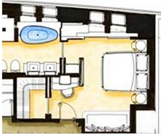
Fig. 50 Cabin desk and chair in VIP Guestroom: walkway is blocked by the desk chair when in use
