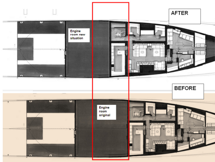
Fig. 30 Above layout is shown of the mega yacht X's bottom deck crew mess, which is extended in dimensions by cutting down in size of the engine room; below picture shows the original layout of the Bottom deck engine room and crew mess
