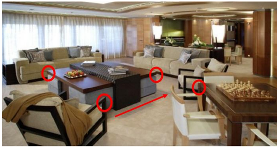
Fig. 55 Upper deck mega yacht X's Saloon; Narrow traffic patterns are shown with interference of furniture
