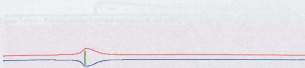
Figure 7.10(e) Steady flow with varying velocity component in the 4 cells above and below the island tip \pm 0.25\% each time step (small random velocity fluctuations mimic the effect of turbulence). Small fluctuations damped by friction ( n = 0.025 \text{ sm}^{-1/3} ).
