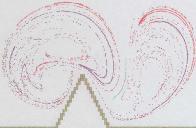
Figure 9.9(c) - Dispersion diagram after 5 complete tidal cycles (released at LW).
