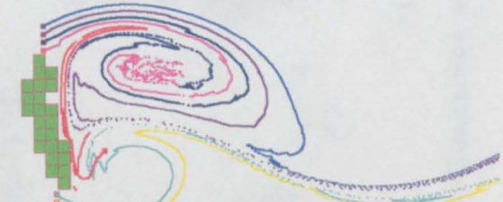
Figure 8.8(e) - Velocity vector plot and particle tracking output at HW (150m mesh).
