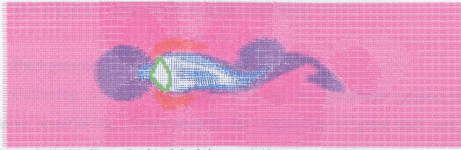
Figure 7.23(a) - Velocity plot of Rupert Bay island simulation at peak tide.
