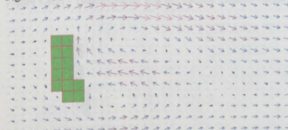
Figure 8.7(f) - Velocity vector plot and particle tracking output at HW+1 (300m mesh).
