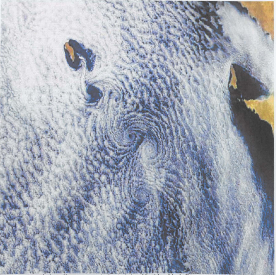
Figure 7.3 – Atmospheric von Karman street wake flow in the lee of Guadalupe Island offshore of Baja, California, USA (20/9/99). Source: http://daac.gsfc.nasa.gov/CAMPAIGN_DOCS/OCDST/vonKarman_vortices.html
