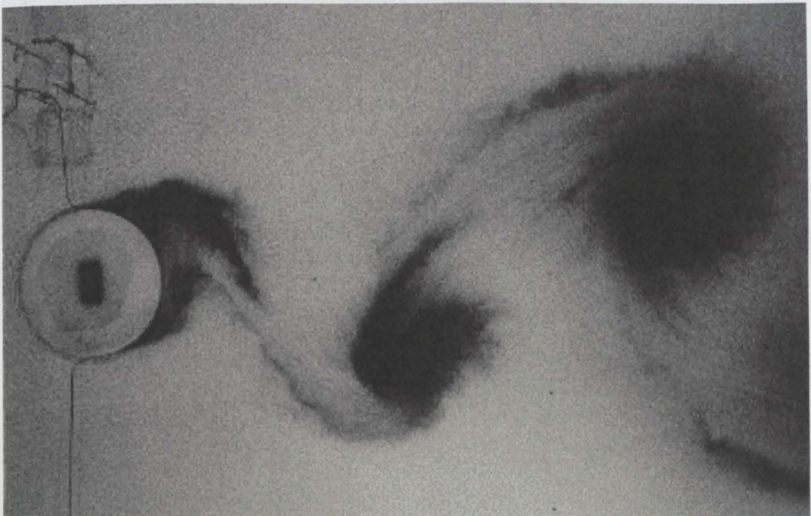
Figure 7.2 – Laboratory von Karman street wake flow. Source: Chen & Jirka (1997)
