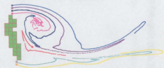
Figure 8.8(c) - Velocity vector plot and particle tracking output at HW-2 (150m mesh).
