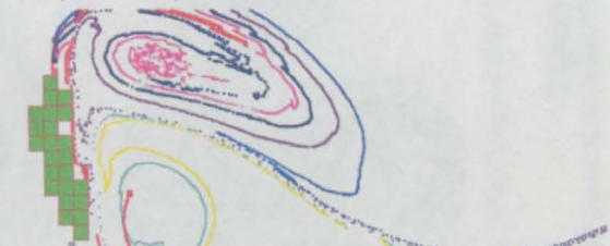
Figure 8.8(f) - Velocity vector plot and particle tracking output at HW+1 (150m mesh).
