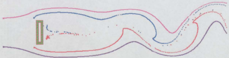
Figure 7.20(a) - Vector plot generated by off-centre position of island feature (interaction with lateral boundary not symmetric).
