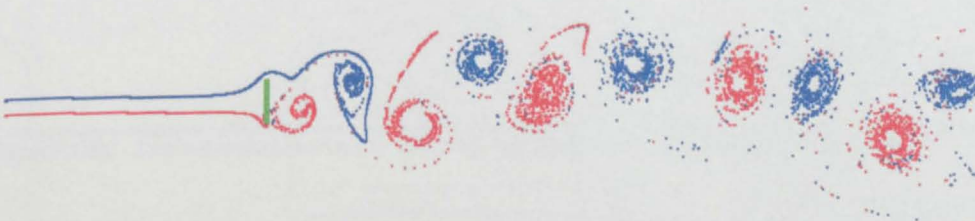
Figure 7.10(d) - Particle tracking output obtained from figure 7.10(c), demonstrating vigorous eddy shedding produced by introducing small random fluctuation into the simulation ( St = 0.183 ).
