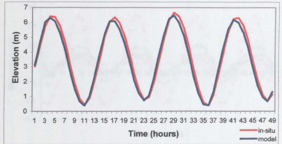
Figure 5.32(d) - Elevation comparison with tidal diamond G.
