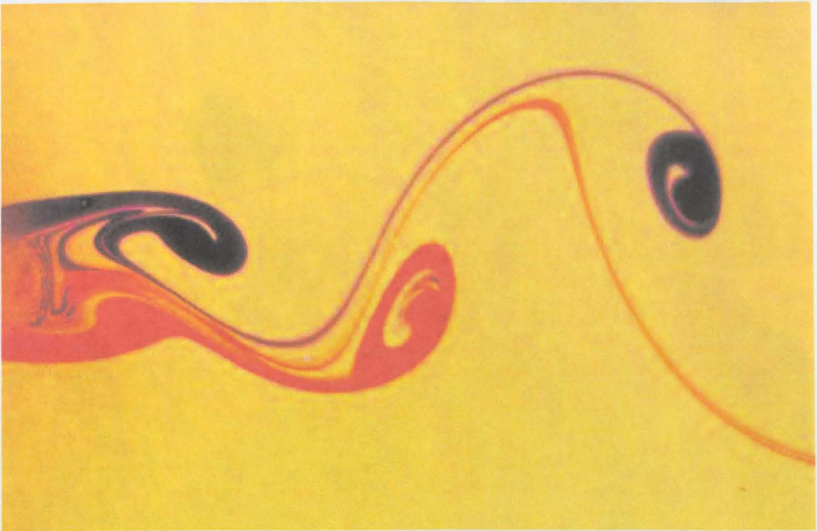
Figure 7.1 – Laboratory von Karman street wake flow. Source: http://www.eng.vt.edu/fluids/msc/gallery/vortex/k_exp.htm
