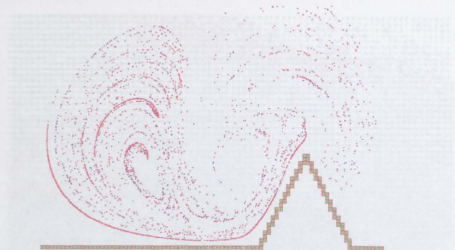
Figure 9.10(b) - Dispersion diagram after 10 complete tidal cycles (released at HW-3).
