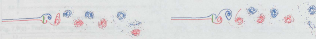
Fig. 7.8(k) - (1300 s) Shed eddies demonstrate significant roll-up. Fig. 7.8(l) - (1400 s).
