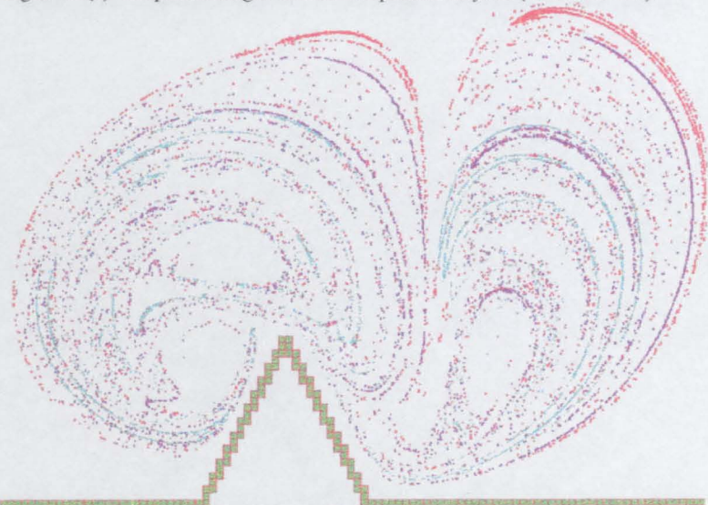
Figure 9.9(d) - Dispersion diagram after 10 complete tidal cycles (released at LW).
