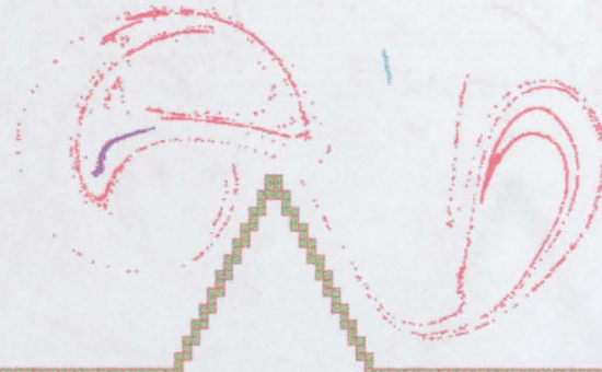
Figure 9.9(b) - Dispersion diagram after 2 complete tidal cycles (released at LW).
