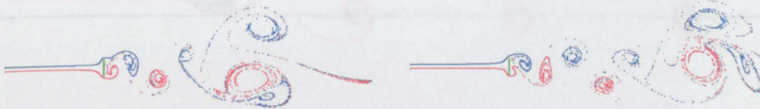
Fig. 7.8(e) - (700 s) Both eddies shed, replacement eddy forming.
