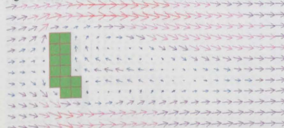
Figure 8.7(e) - Velocity vector plot and particle tracking output at HW (300m mesh).
