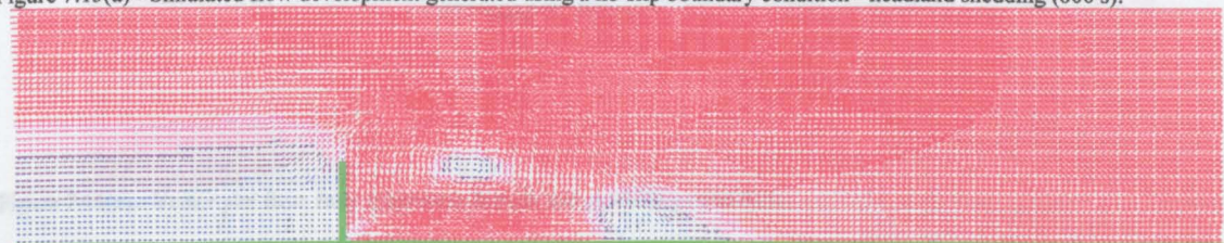
Figure 7.13(b) - Simulated flow development generated using a free-slip boundary condition - standing eddy (no shedding) (600 s).
