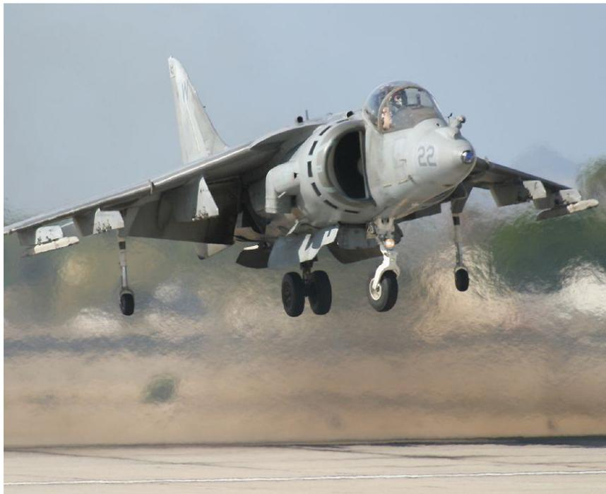
**Figure 1.1 – BAE Harrier during vertical takeoff ©<http://www.richard-seaman.com/>.**
