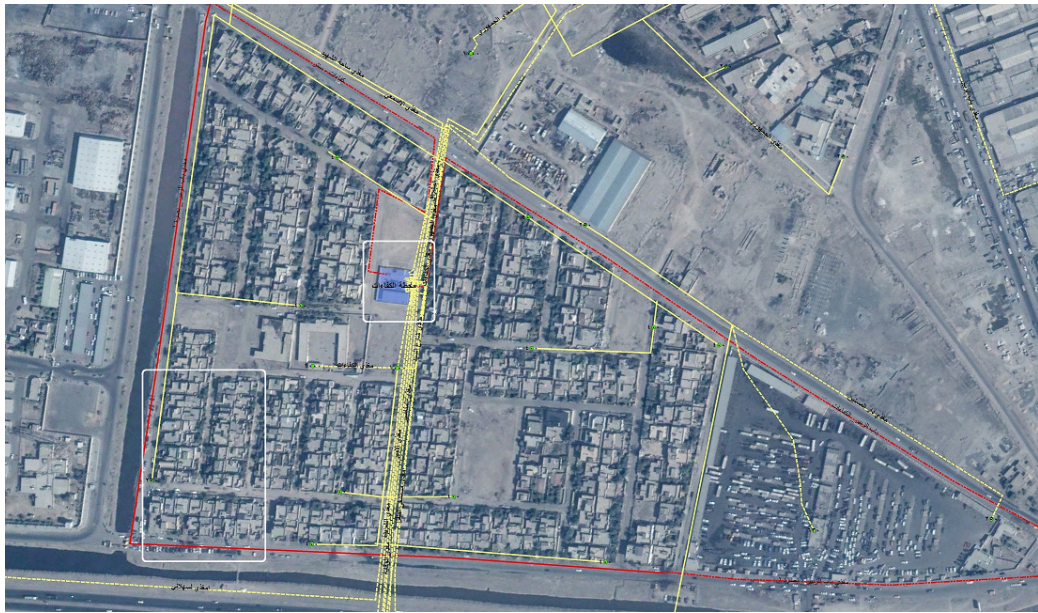
Figure 5.9: Kafaat Substation and accompanying LVDN.
