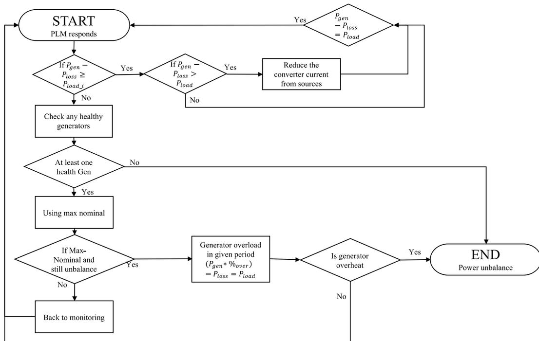
**Figure 53. PLM with only Generator overload**
