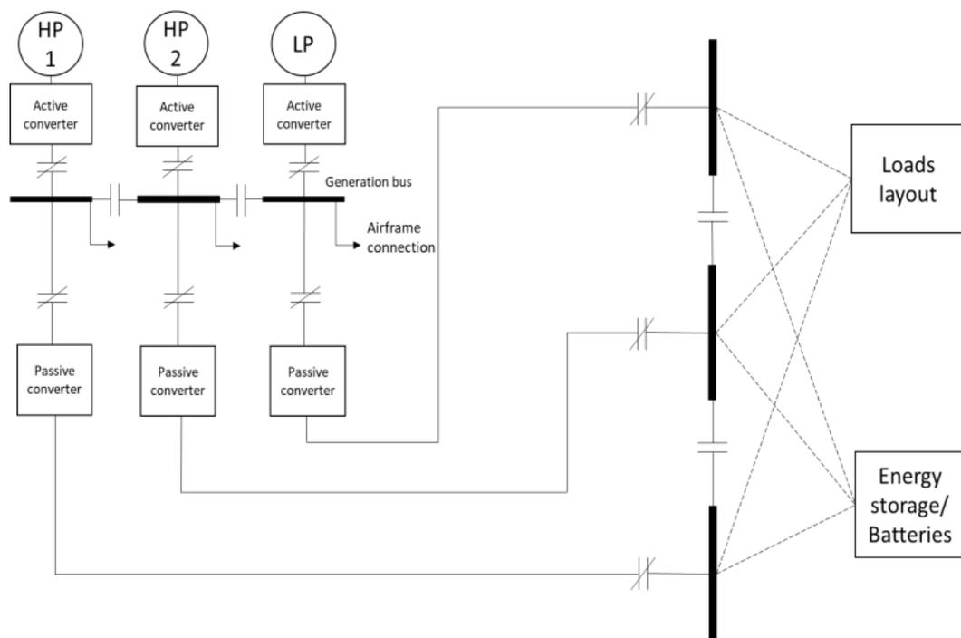
**Figure 13. Three-channel architecture with sectionalised bus arrangement**
