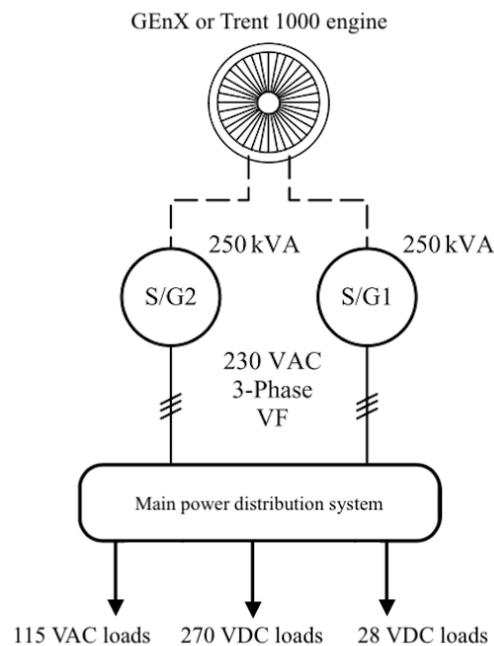
Figure 8. Boeing 787 engine power architecture [29]
