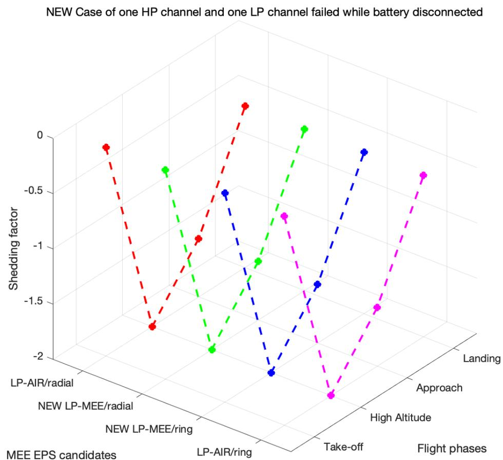
**Figure 45. The new LP-MEE series concept has the same LSF as the LP-Air series concept**
