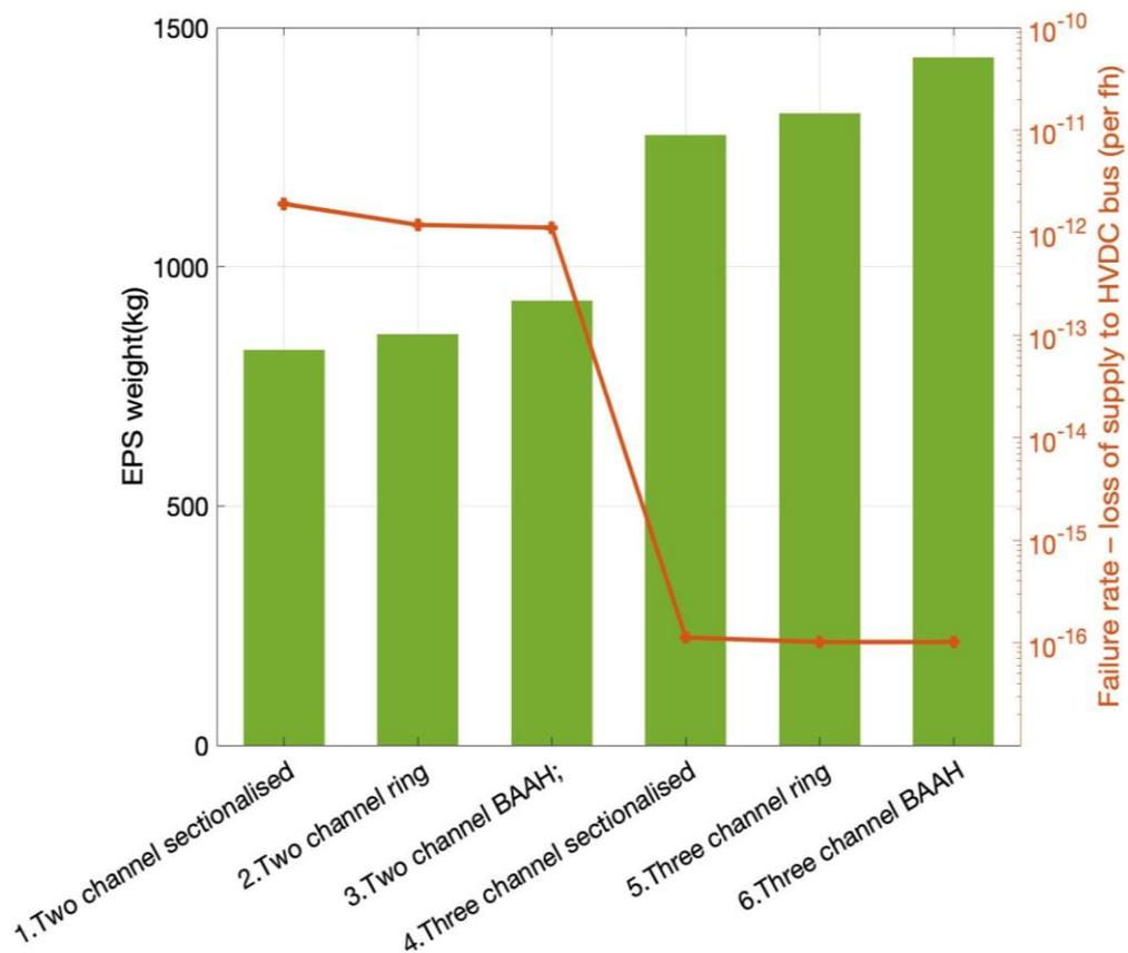
Figure 17. Reliability of power distribution architectures
