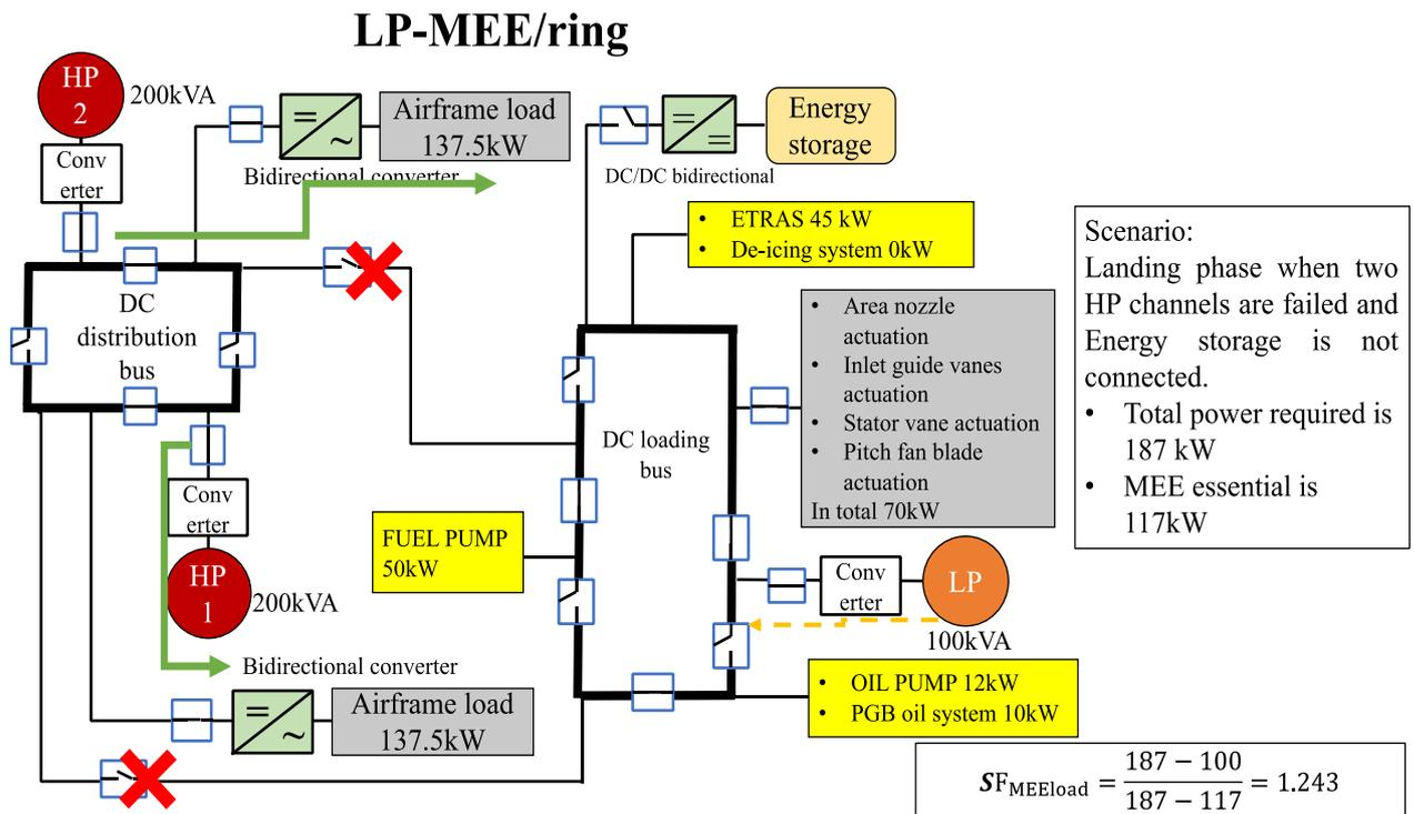
**Figure 39. An example of the power reconfiguration case study**
