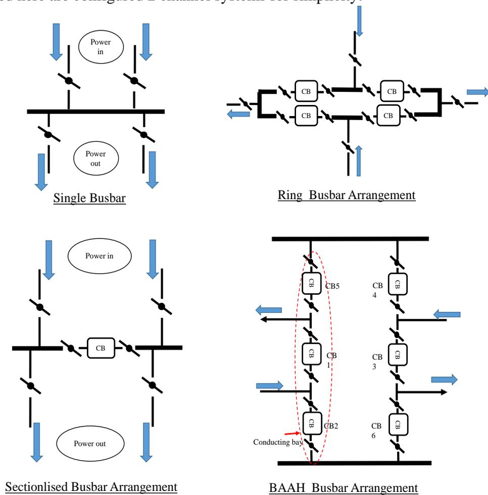
**Figure 21. Candidate busbar topologies for the MEE BPA**
