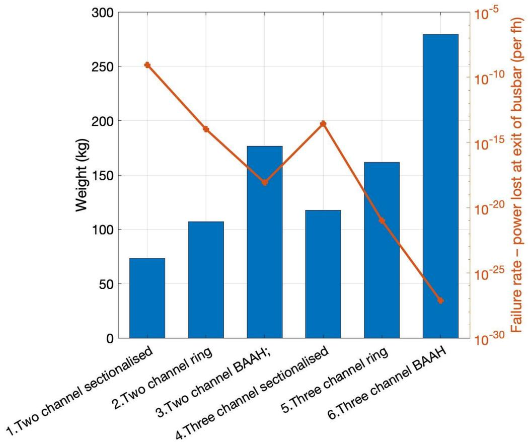
Figure 16. Busbar failure rates and weight
