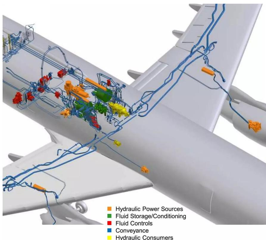
**Figure 7. Hydraulic architecture of a commercial aircraft [36]**
