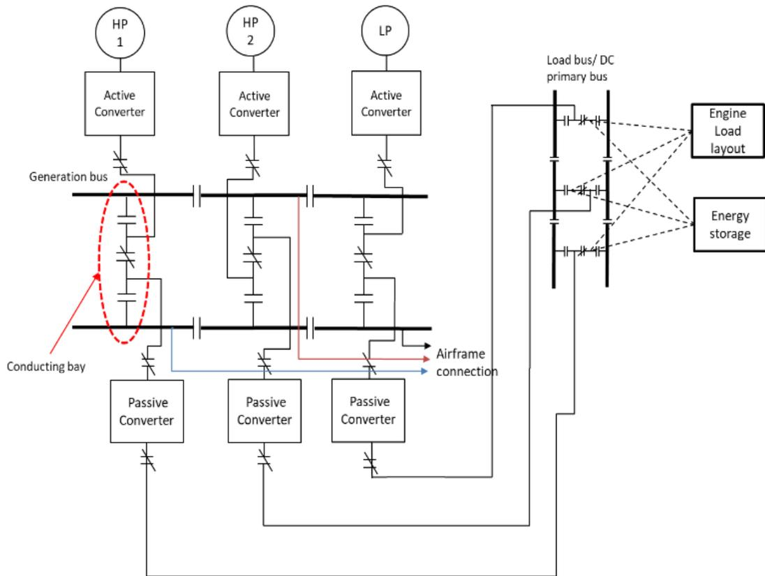
**Figure 15. Three-channel architecture with breaker and a half bus configuration**
