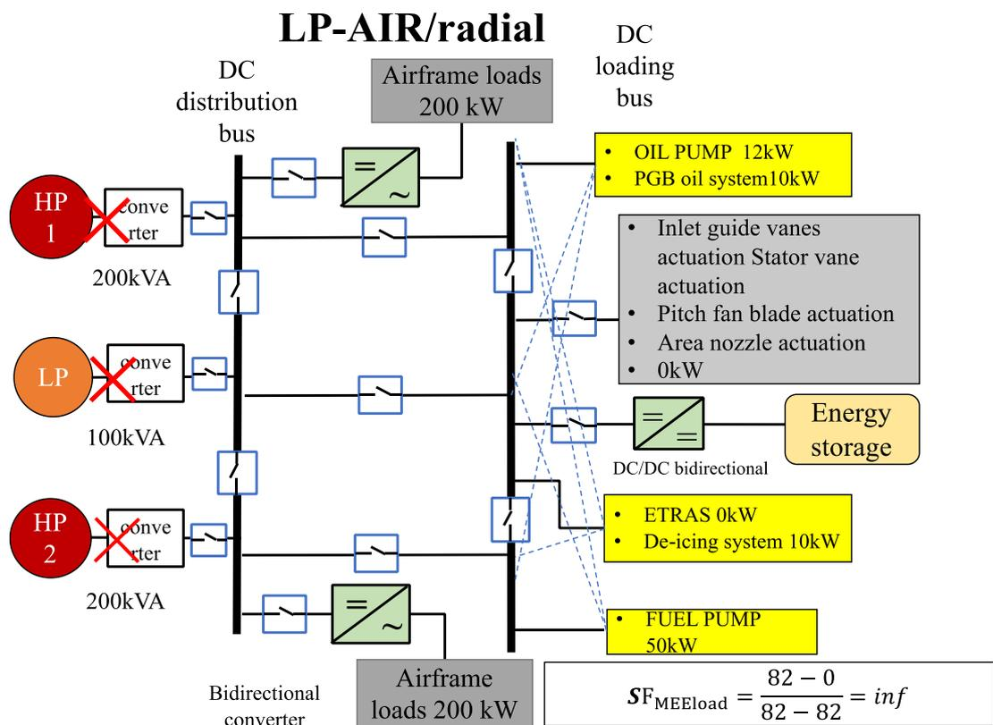
The EPS concepts that selected by parameter classification optimisation can easily ride through the single failure modes via coordinate with proper power management. If extreme cases occurred such as all generator failed at the same time, there are no many supply flexibilities can be operated in the power architecture. However, the interesting design optimisation/enhancement lies in the failure mode of two channels. The design
