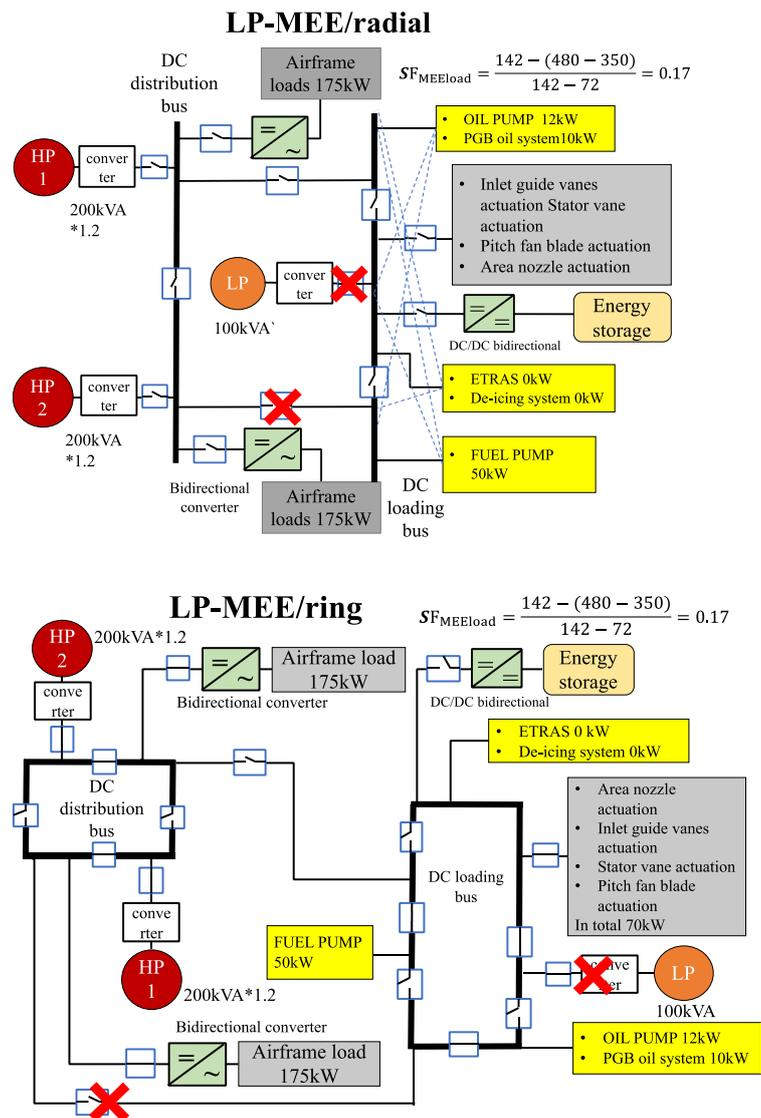
**Figure 64. EPS concepts under One HP channel + One LP channel failure mode with PLM option: ESS and load shedding and 120% generator overload at Take-off Phase.**
