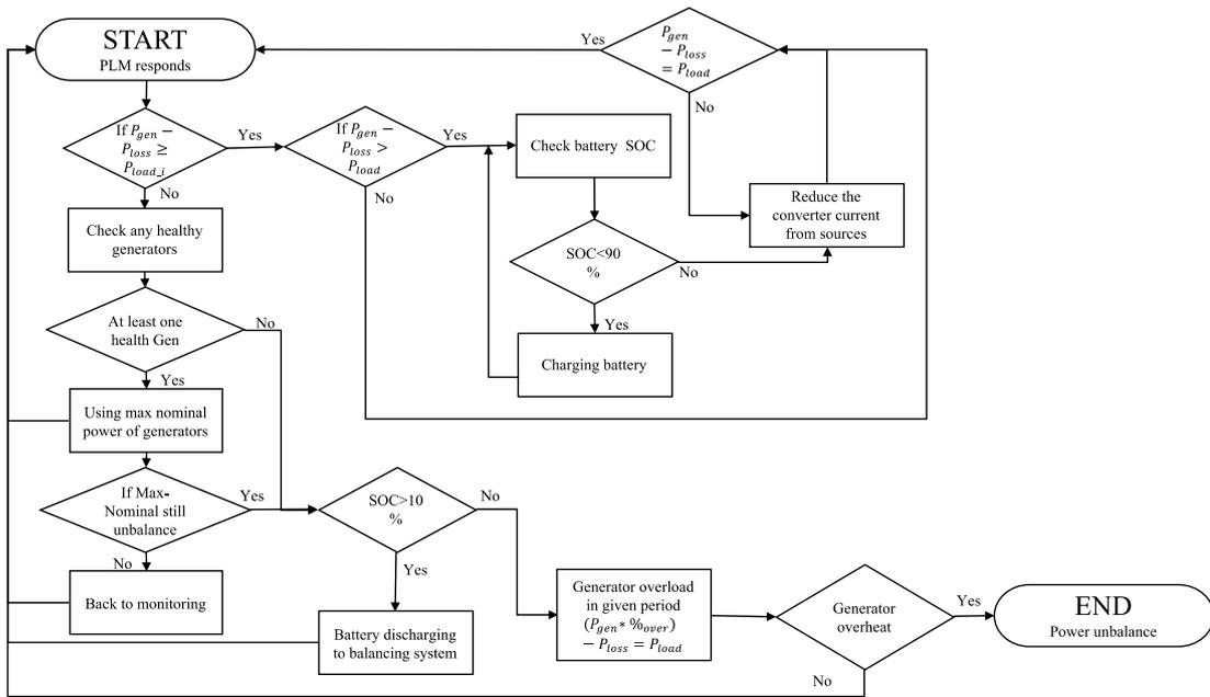
Figure 56. The PLM scheme with ESS and generator overload
