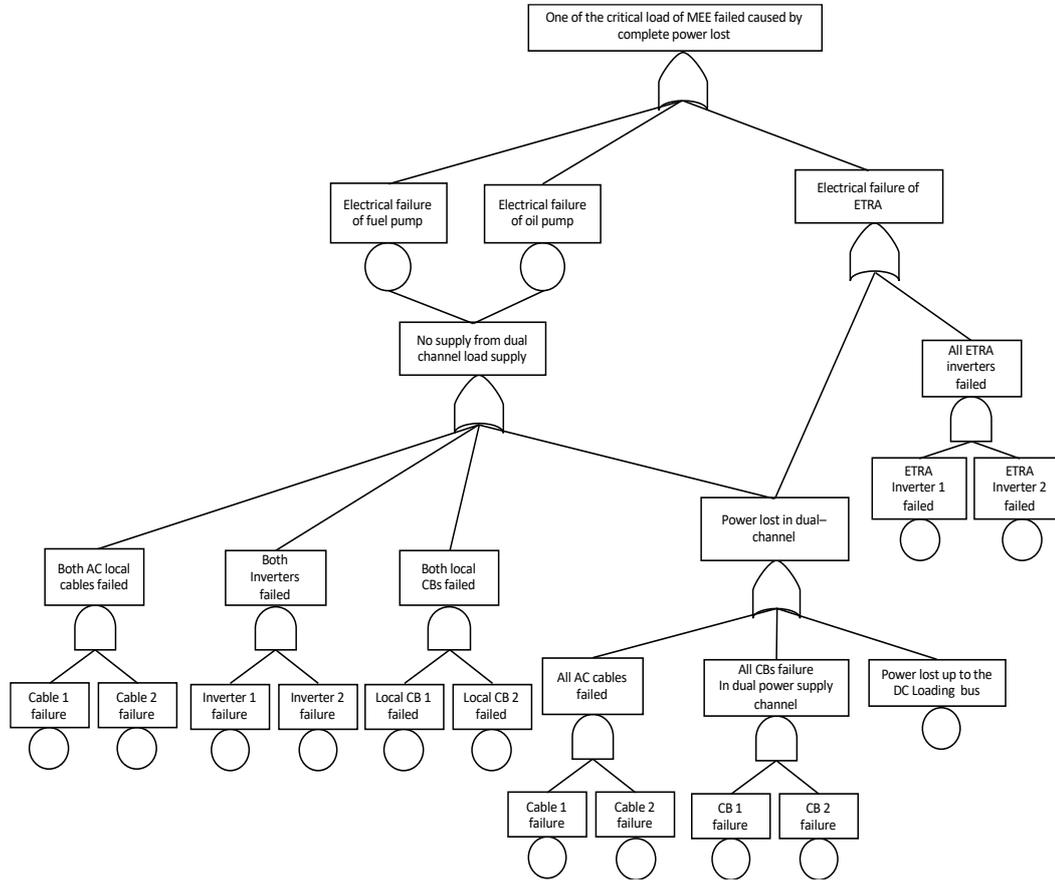
**Figure 19. Fault tree analysis on power flow of the essential loads section of MEE with a Dual-channel architecture, executed by Mobius software [58]**
