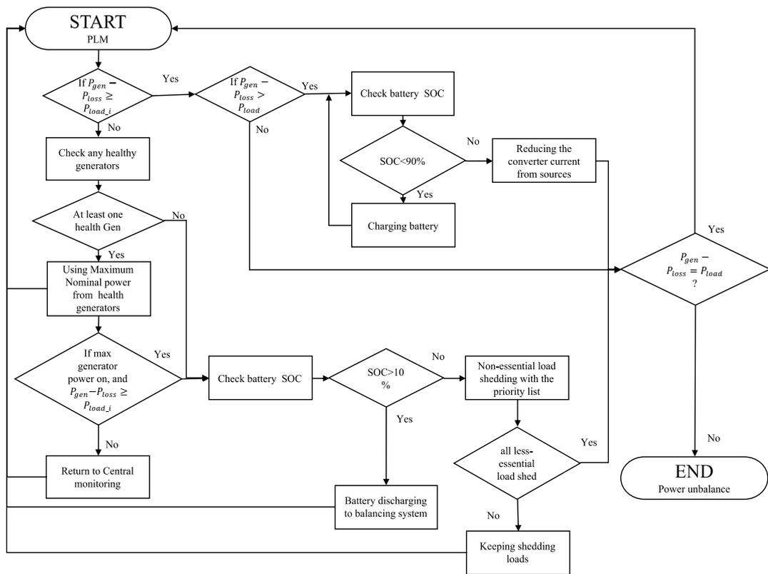
**Figure 55. PLM scheme with ESS and load shedding**
