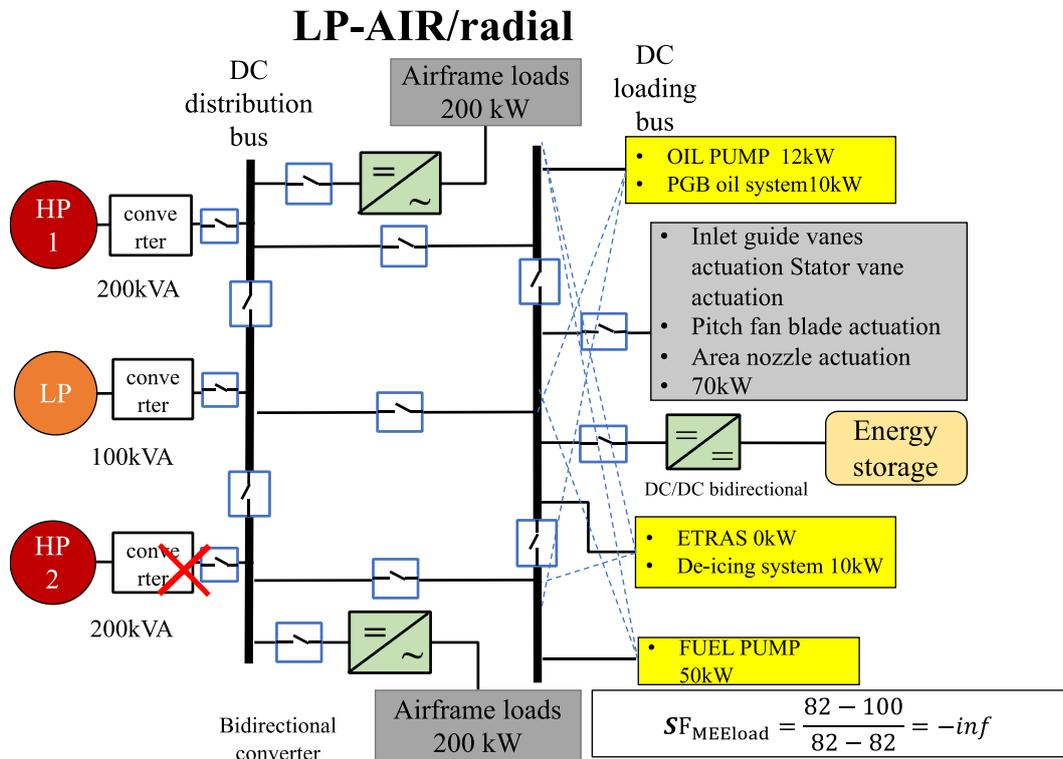
**Figure 59. One HP generator failed in cruise phase**
