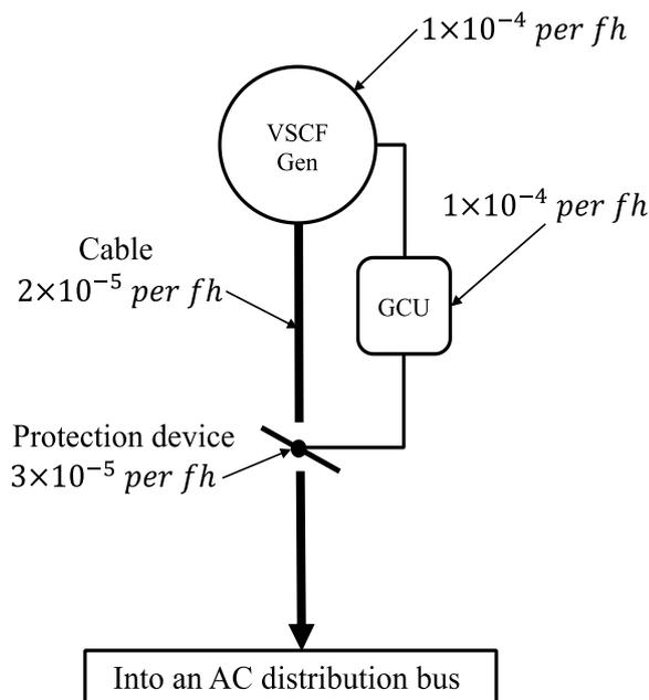
**Figure 20. The VSCF generation system with component failure rates.**
