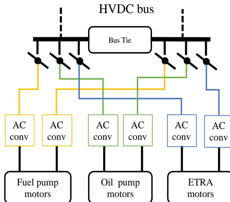
Figure 22. MEE essential loads redundancy
