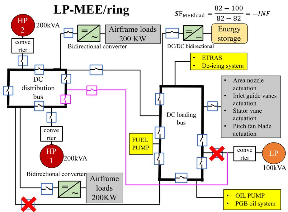
**Figure 66. The improved EPS concepts under One HP channel + One LP channel failure mode with PLM option: ESS and load shedding at High Altitude Phase**
