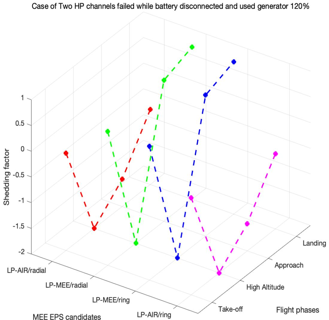
**Figure 41. Using generator overloading in the power management strategy and SF below one**
