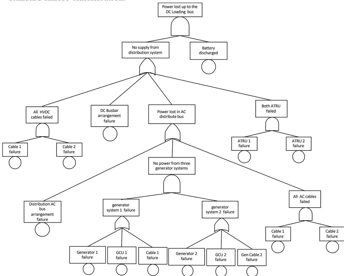
**Figure 18. Fault tree analysis of the distribution system of MEE with a Dual-channel architecture, executed by Mobius software [58]**
