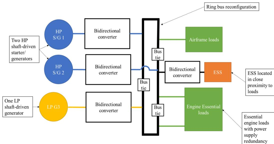
**Figure 23.**The example of baseline power architecture for MEE
