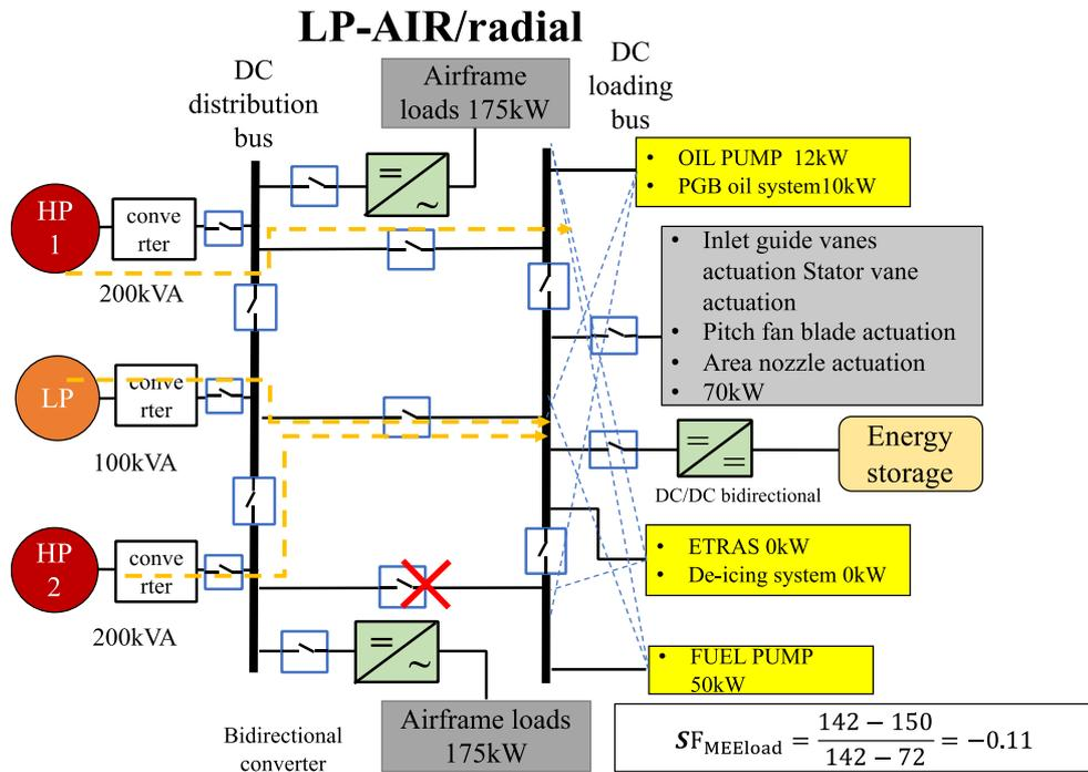
**Figure 58. Single channel failure in take-off phase**
