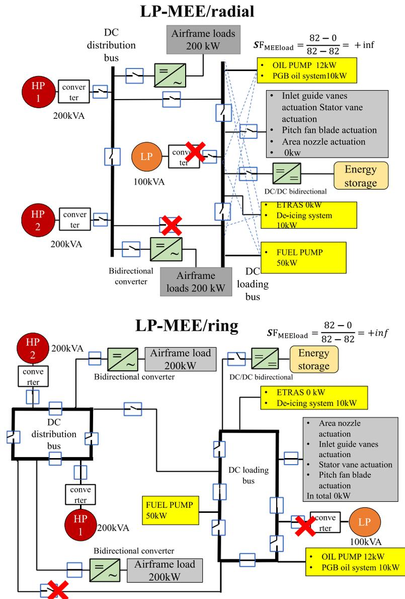
**Figure 65. EPS concepts under One HP channel + One LP channel failure mode with PLM option: ESS and load shedding at High Altitude Phase**
