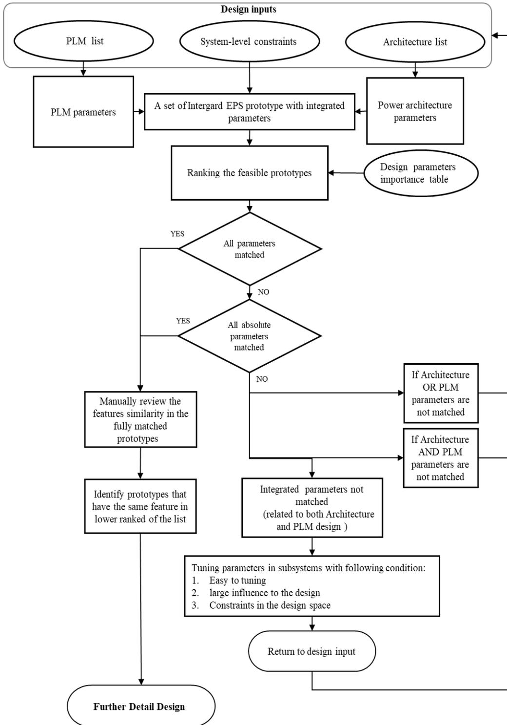
Figure 25. Detail flow chart of parameter classification for optimising the integrated MEE features
