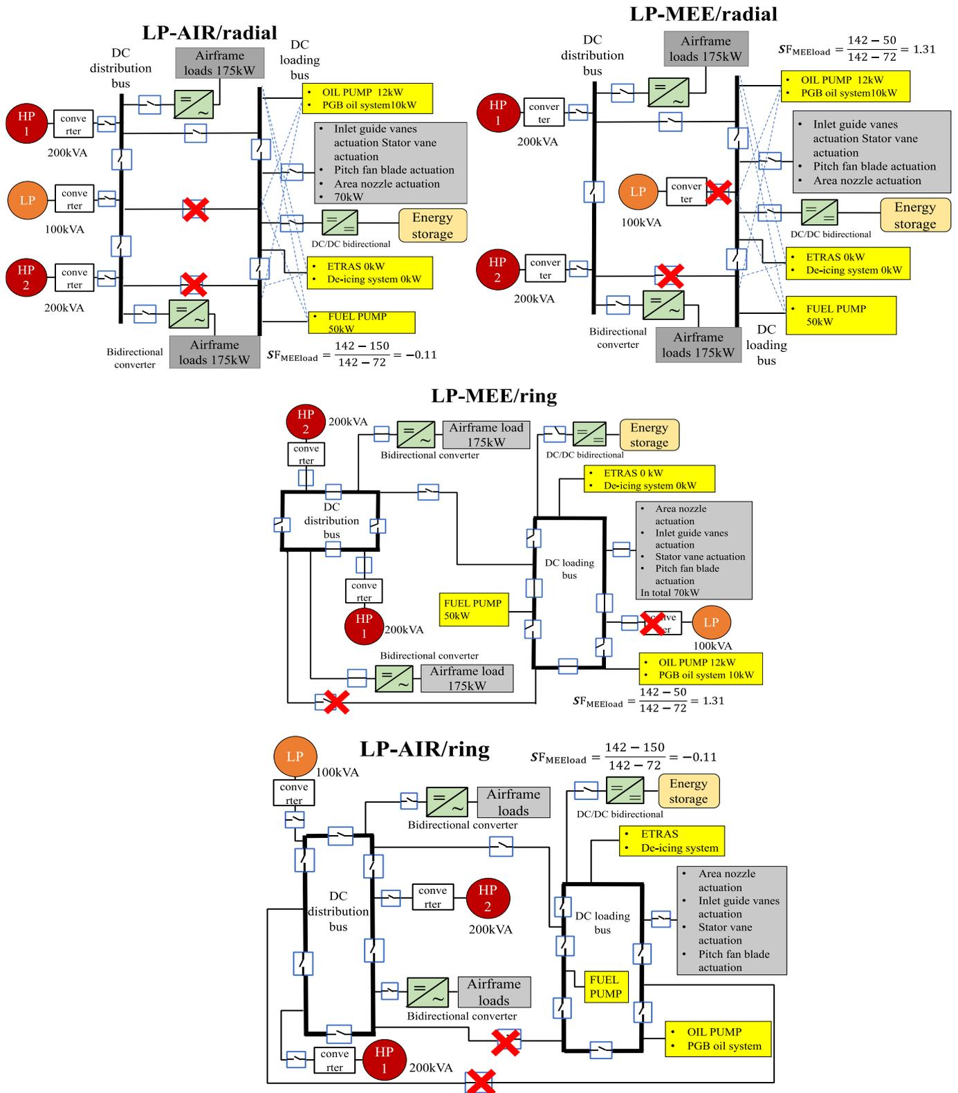
Figure 63. EPS concepts under One HP channel + One LP channel failure mode with PLM option: ESS and load shedding at Take-off Phase
