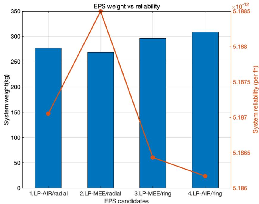
**Figure 38. The MEE power architecture weight vs system reliability**
