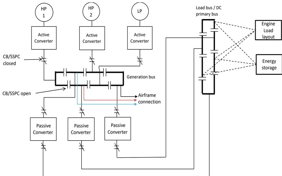
**Figure 14. Three-channel architecture with ring bus configuration**
