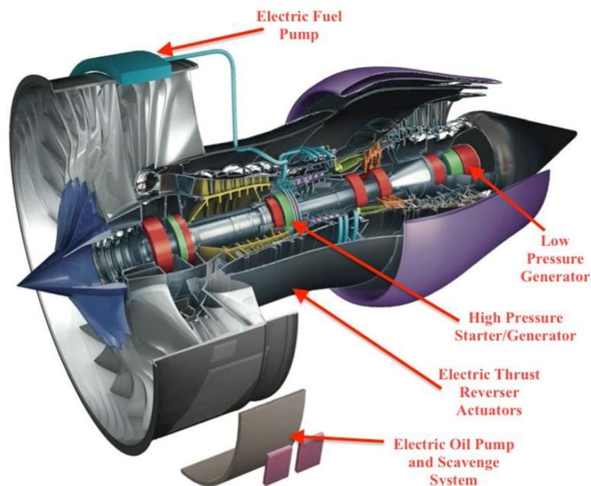
Figure 6. MEE concept that proposed by Rolls Royce [35]
