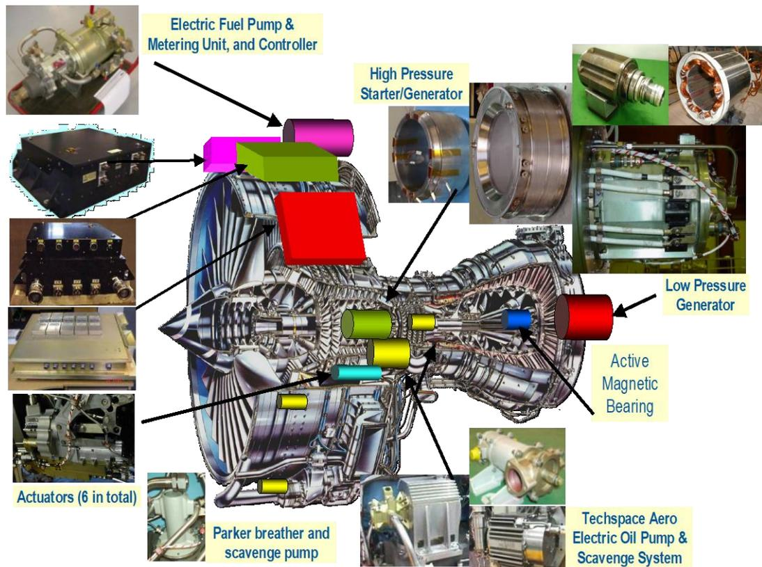
**Figure 5. Concept of MEE form ESVR demonstrator [31]**
