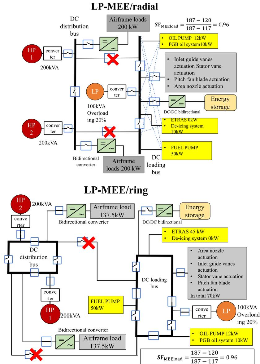
**Figure 62. EPS concepts under two HP channel failure mode with PLM option: ESS and load shedding and 120% generator overload at Landing Phase.**
