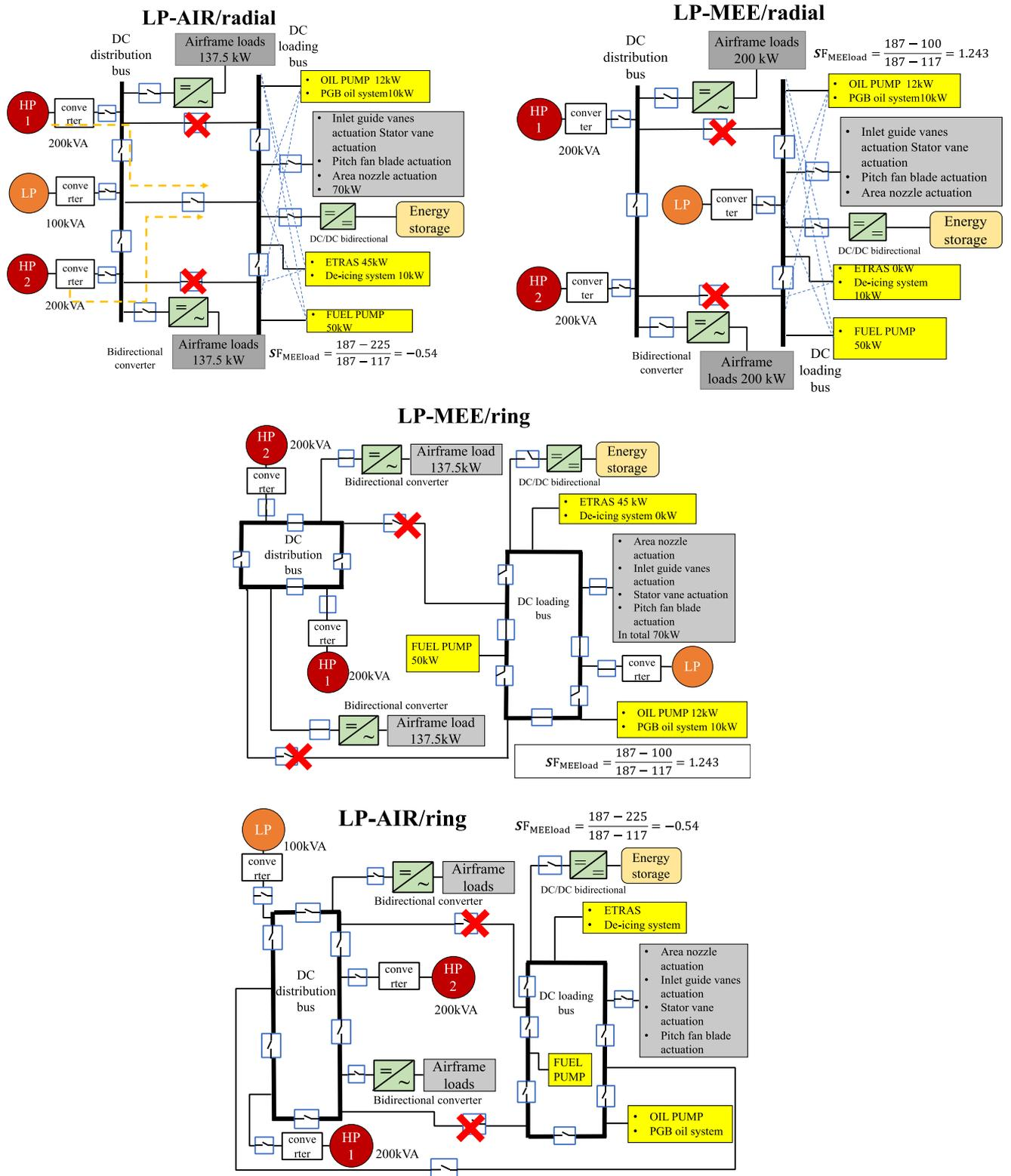
Figure 61. EPS concepts under two HP channel failure mode with PLM option: ESS and load shedding at Landing Phase
