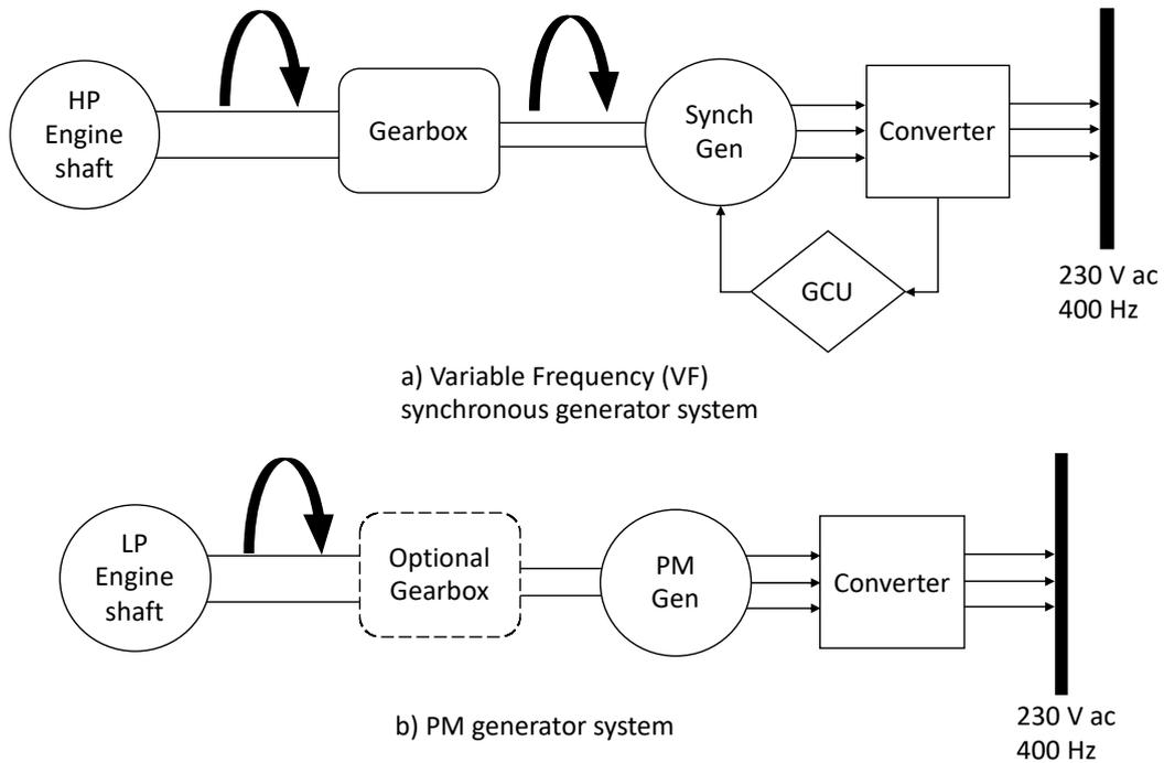
Figure 12. Different types of MEE generator system
