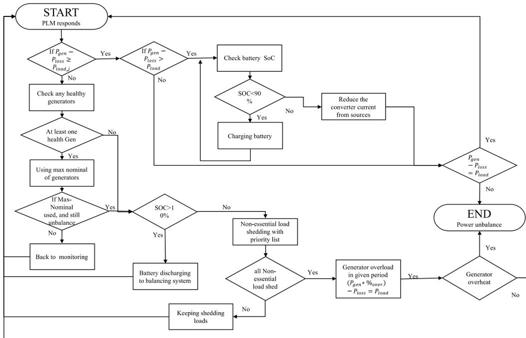
Figure 57. PLM scheme with ESS, shedding and generator overload
