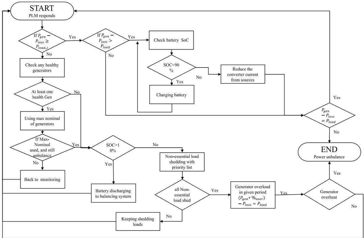
**Figure 37. PLM strategy with ESS, Load shedding and Generator overloading**
