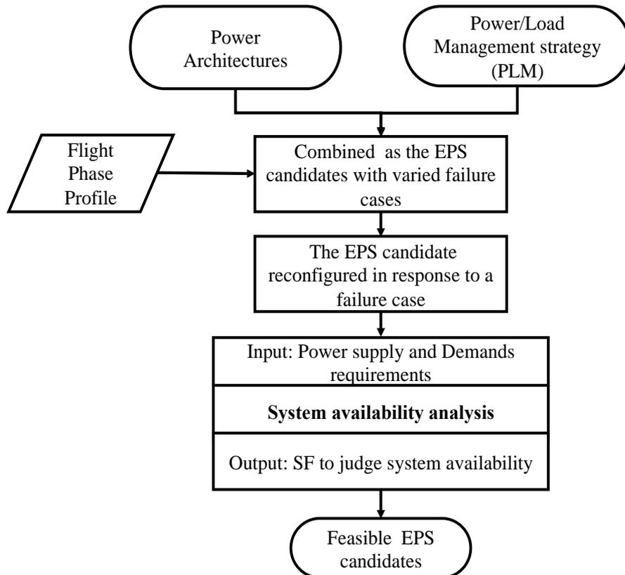
Figure 33. System availability analysis via a co-synthesis process
