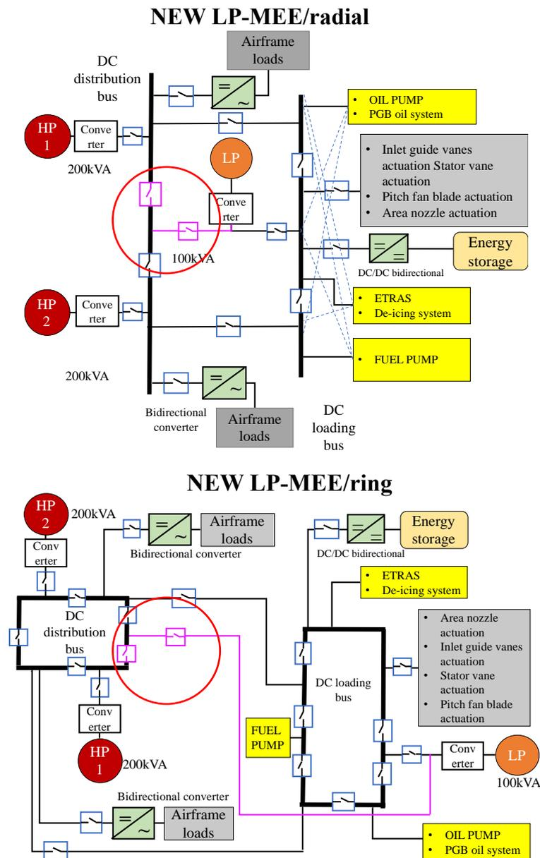
Figure 44. Two new EPS options based on LP-MEE/radial and LP-MEE/ring
