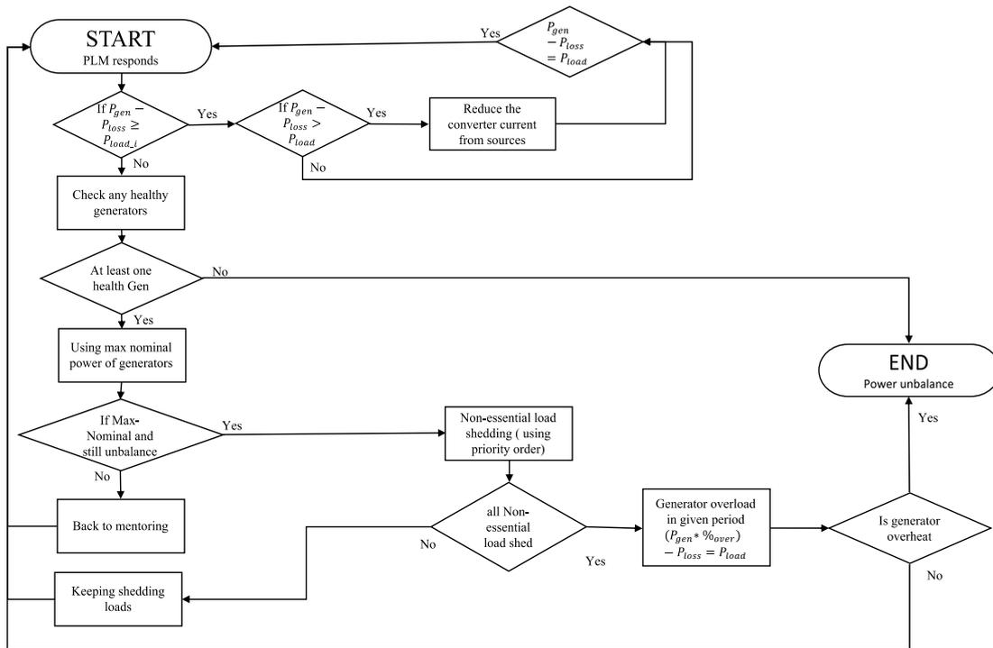
**Figure 54. PLM scheme with shedding and generator overload**
