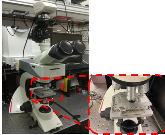
Figure 3.1: High throughput optical microscopy system with a close up section of the nanometer stage sample holder
