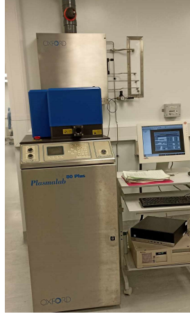
Figure 2.6: Plasma Enhanced Chemical Deposition machine used in this thesis.
