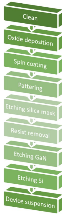
Figure 2.2: Flow chart of the fabrication of suspended membrane arrays
