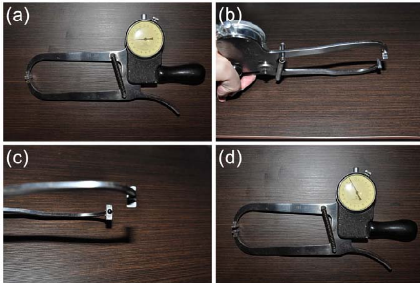
Figure 5-3 Thickness gauge modification
