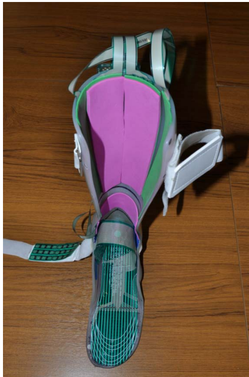
Figure 3-9 EVA foam sheet applying on the sensor at the defective positions
