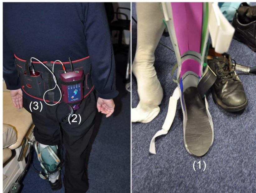
Figure 3-10 pedar ® -x system: (1) pedar ® -x insole, (2) Bluetooth ™ telemetry system, (3) rechargeable NiMH battery
