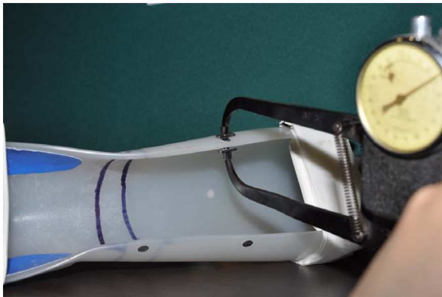
Figure 5-4 The AFO thickness measurement set up
