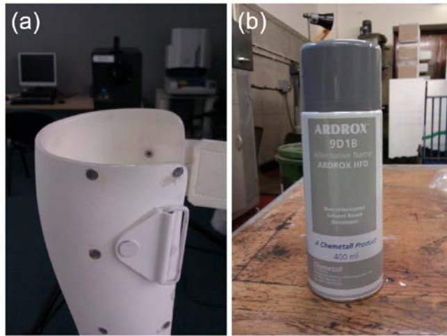
Figure 4-2 (a) powder sprayed on AFO surface and (b) Ardrex 9D1B
