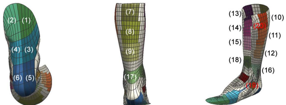
Figure 5-7 Locations of loads applied on FE model of AFO
