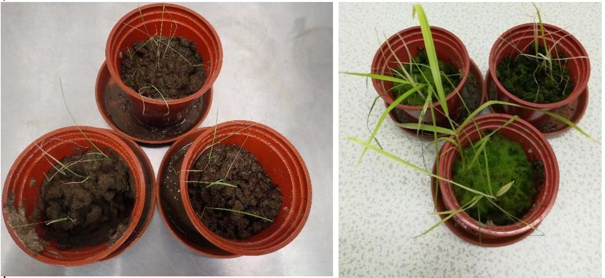
**Figure 36** Five RCG plants grown per pot in pot trials over 10 weeks in an unamended mine soil (WH3) (left) and a soil (WH3) amended with 30% green waste compost (right)
