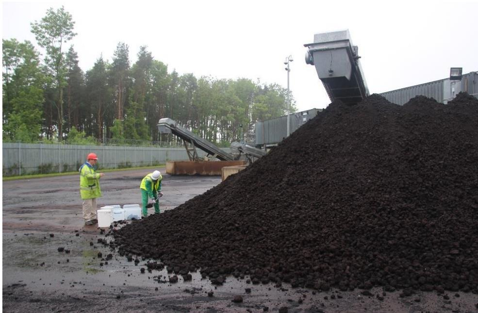
**Figure 32** Collection of drinking water treatment residue bulk sample from Mosswood water treatment works (Northumbrian Water Ltd.).
