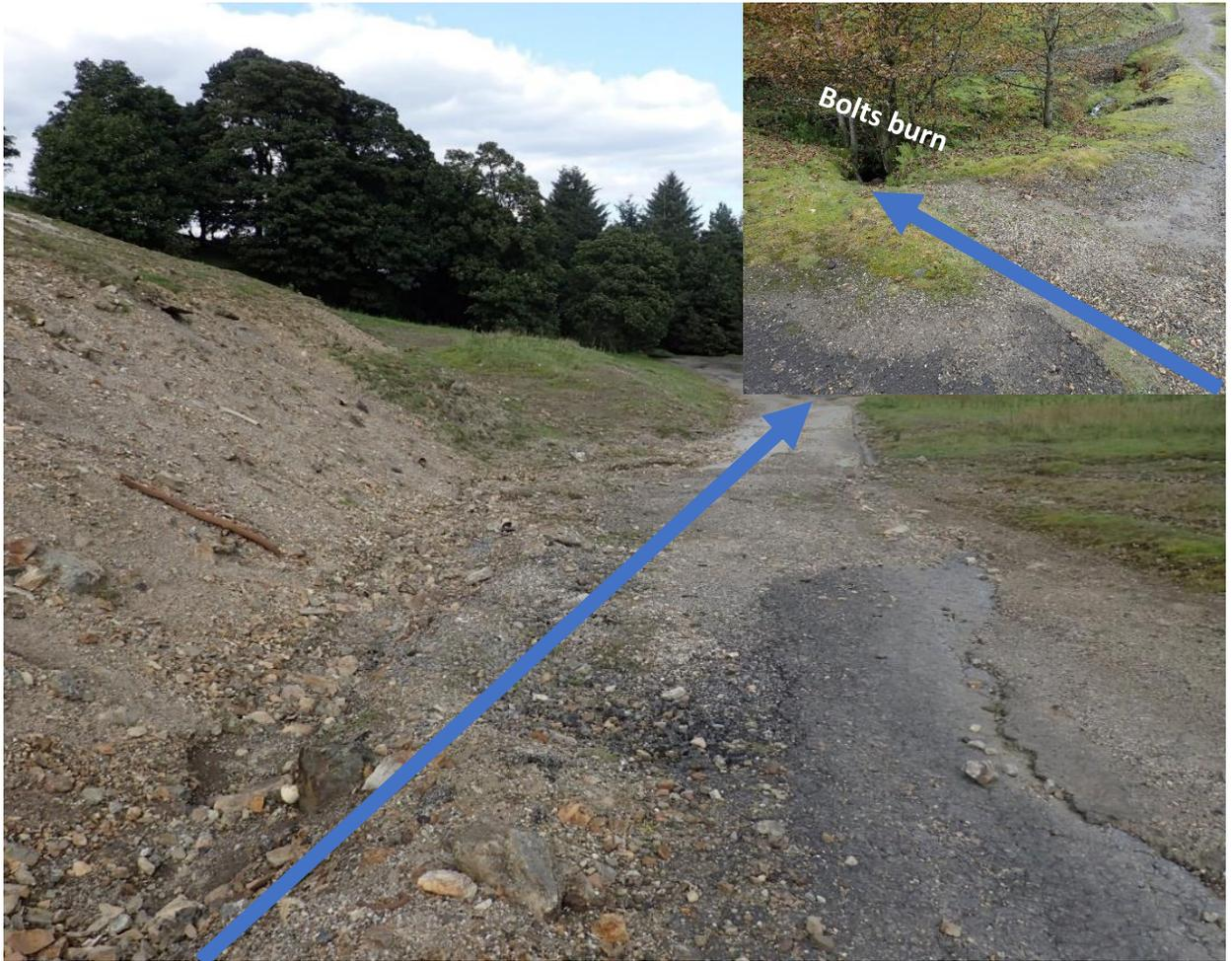
**Figure 30 Evidence of erosion and run off from Whiteheaps mine site into Bolts Burn, resulting from the movement of water due to rainfall. Blue arrows show noted direction of travel of eroded sediment (February 2020)**
