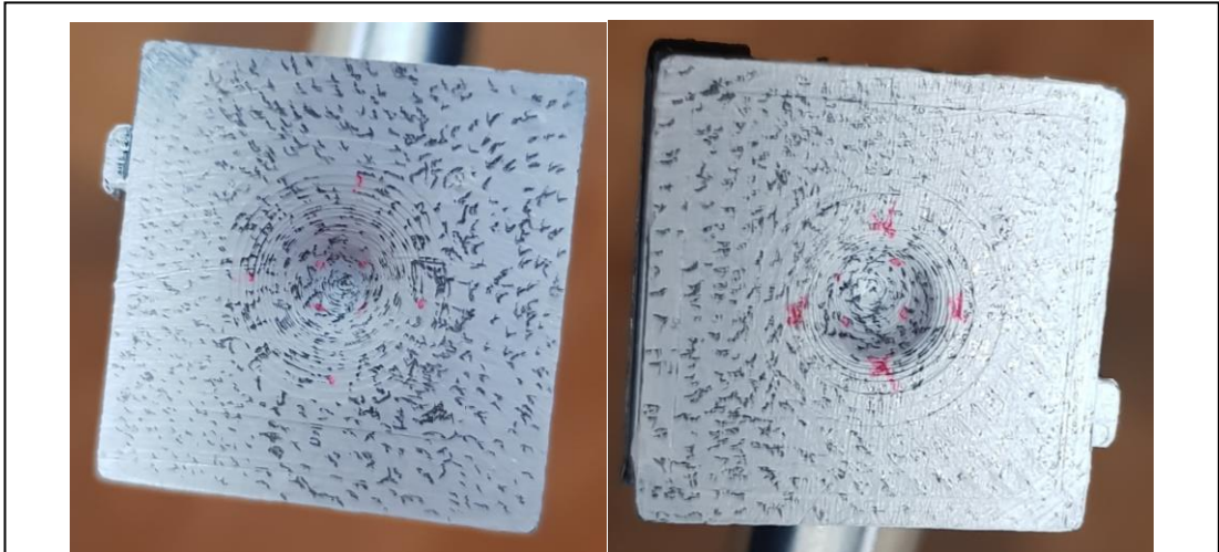
Figure 81: Images taken of the normal (LEFT) and glaucomatous (RIGHT) ONH targets, showing the speckle pattern applied, for ground truth scanning.
