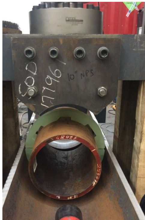
Figure 8.5: Experimental setup for the centraliser testing; showing the circular loading bracket at the top and the inner pipe and partial outer pipe, both of which act as supports for the centraliser during testing.
