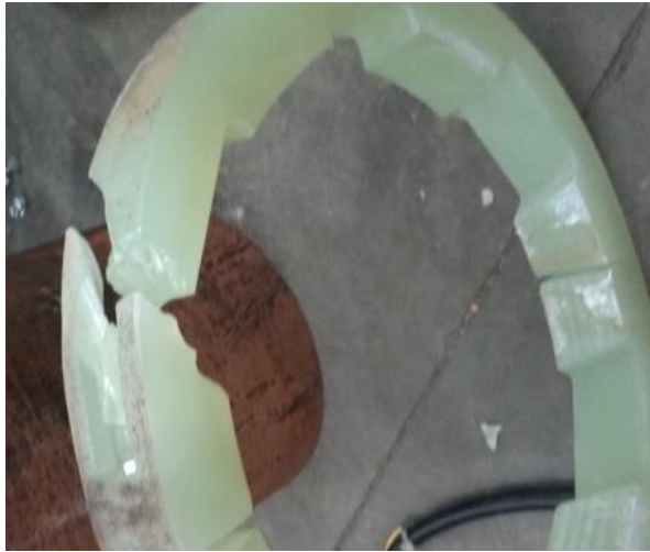
Figure 8.2: Image of the failed centraliser, showing that it has broken at the heating wire cut out
