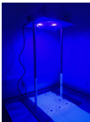
Figure 5.17 Experimental set-up for exposure of seeded surface coupons using miniaturised 405-nm light EDS.
