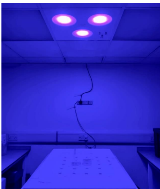
Figure 4.7 405-nm light EDS exposure of surface-seeded pathogens in ‘blue-only’ mode at a distance of ~1.5 metres from the light source, providing an irradiance at the sample surface of 0.5 mW cm -2 .
