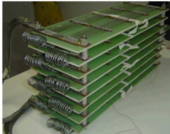
Figure 2- A modular SFCL consisting of 16 elements; each containing 4 YBCO tapes of 0.4 m length with shunt protection [14]
