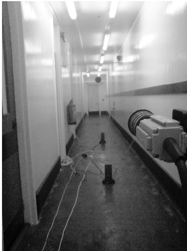
Figure 3.13. Photograph of the corridor in which flight tests were conducted, showing video camera, antennas and circular target.
