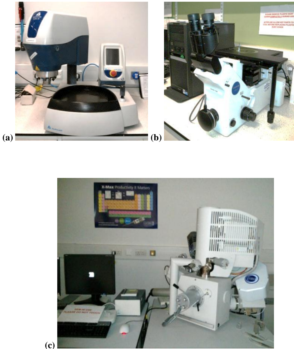
Fig. 3.6. Equipment used for sample preparation and microstructural characterisation of specimens: (a) Buehler EcoMet 300 Pro Grinder-Polisher; (b) Olympus GX51 optical microscope; (c) Quanta FEG 250 scanning electron microscope.
