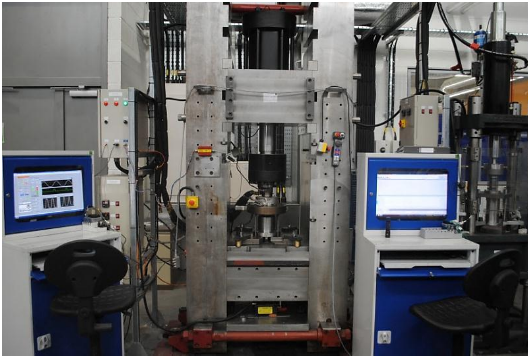
Fig. 3.1. Hydraulic press used in this work for I-ECAP experiments.
