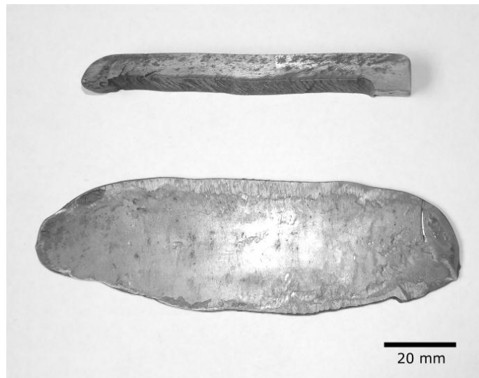
Fig. 6.4. Samples after four passes of I-ECAP (upper) and I-ECAP followed by side upsetting (lower).
