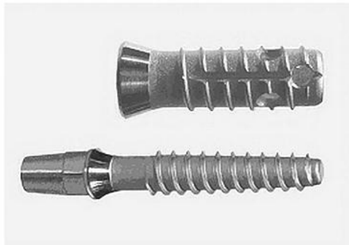
Fig. 2.3. Dental implants made of nanostructured Ti. Image was taken from the work by Valiev et al. (2008).
