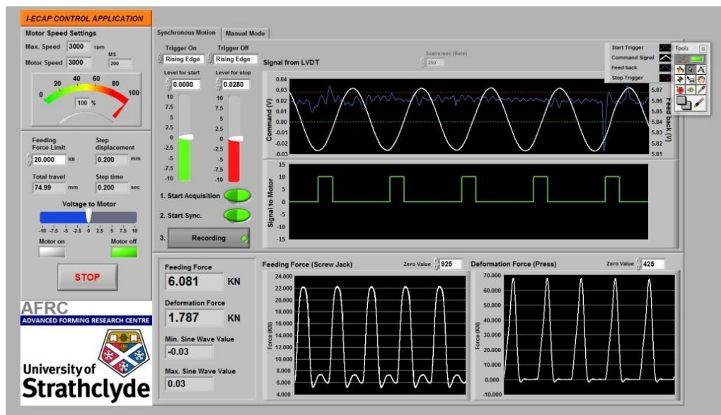
Fig. 3.3. Screenshot from NI application used to control feeding of billets.
