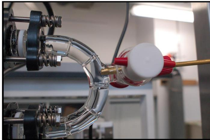
**Figure 5.30: Adapted bend for in-line PAT.** Photograph showing a standard COBC bend modified with a minimised dead volume key tap adaptor and an ATR-FTIR probe inserted.
