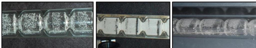
**Figure 6.13: Encrustation patterns on a DN15 COBC glass straight.** Photographs illustrating an alternating ring pattern of encrusted LGA during MFOBC crystallisations.
