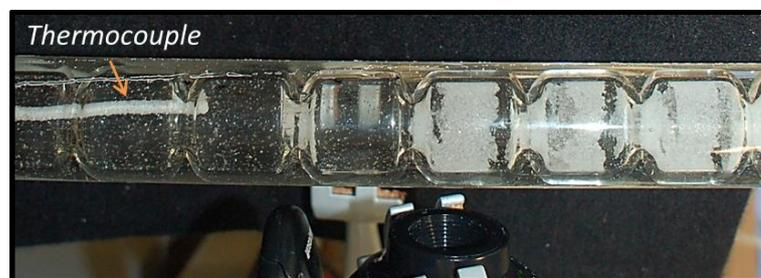
**Figure 6.16: Sacrificial encrustation.** Photograph showing encrustation along the COBC straight of a MFOBC. Image shows preferential encrustation on the stainless steel thermocouple (left) and in area where the thermocouple is not present (right) dominant encrustation on the vessel walls.
