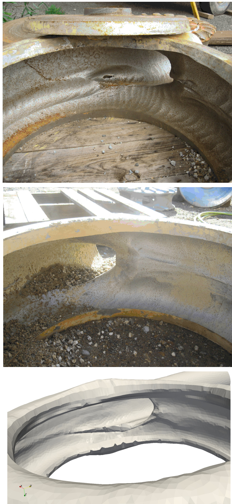
Figure 6.63: Top: 86AH centrifugal slurry pump's volute operating with Impeller WRT1, Middle: Picture of 86AH centrifugal slurry pump's volute obtained from worn unit operating with F6145WRT1 impeller and F6083 throatbush, Bottom: Computational volute wall deformed according to erosion showing similar erosion pattern
