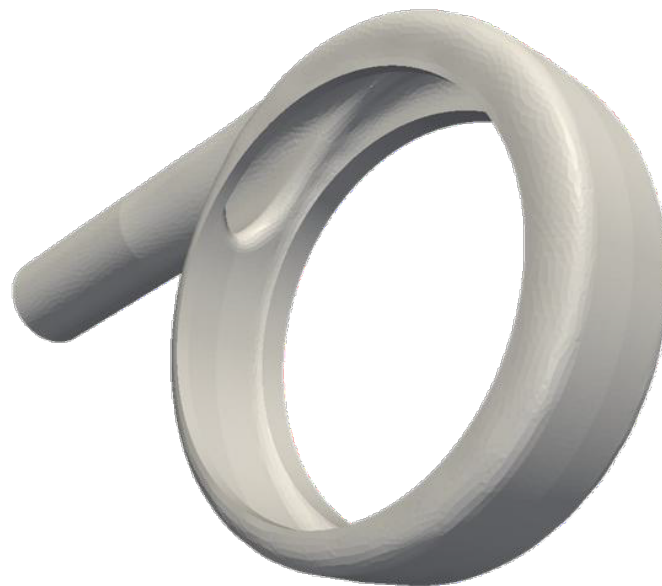
Figure 6.59: Picture of 86AH centrifugal slurry pump's volute
