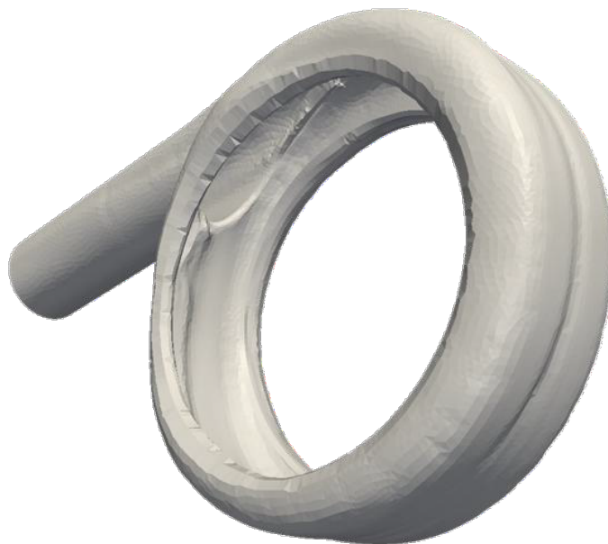
Figure 6.61: Picture of 86AH centrifugal slurry pump's volute deformed according to erosion
