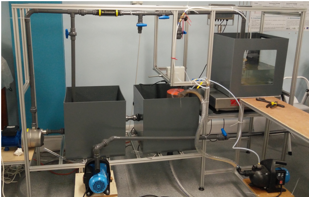
Figure 5.10: Test rig with sacrificial pump, scale and stirrer
