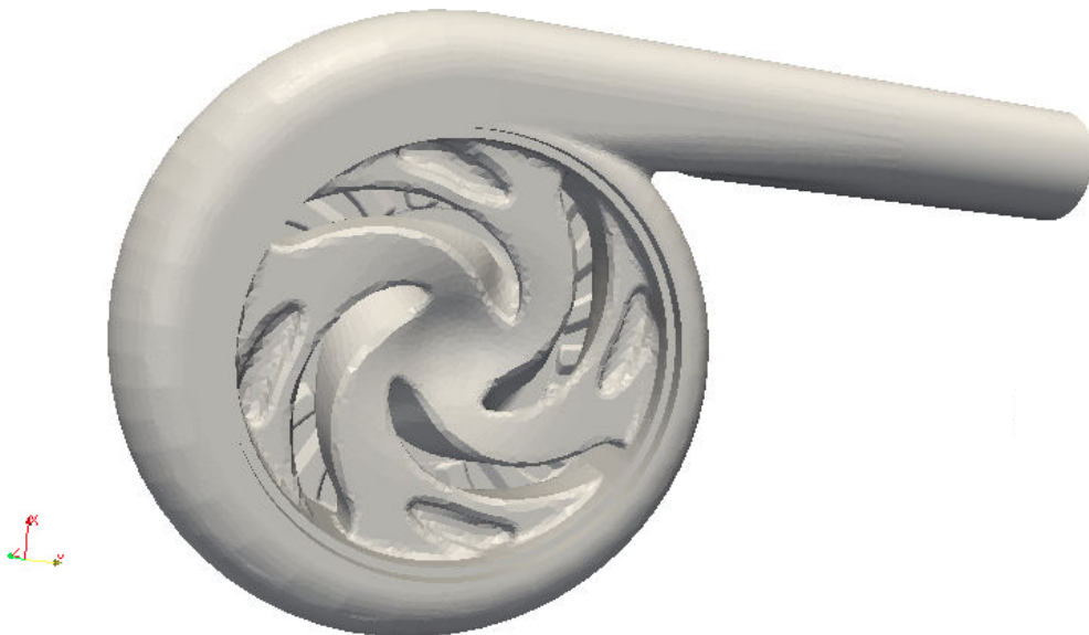
Figure 6.65: Picture of 150WBH centrifugal slurry pump showing uneroded impeller
