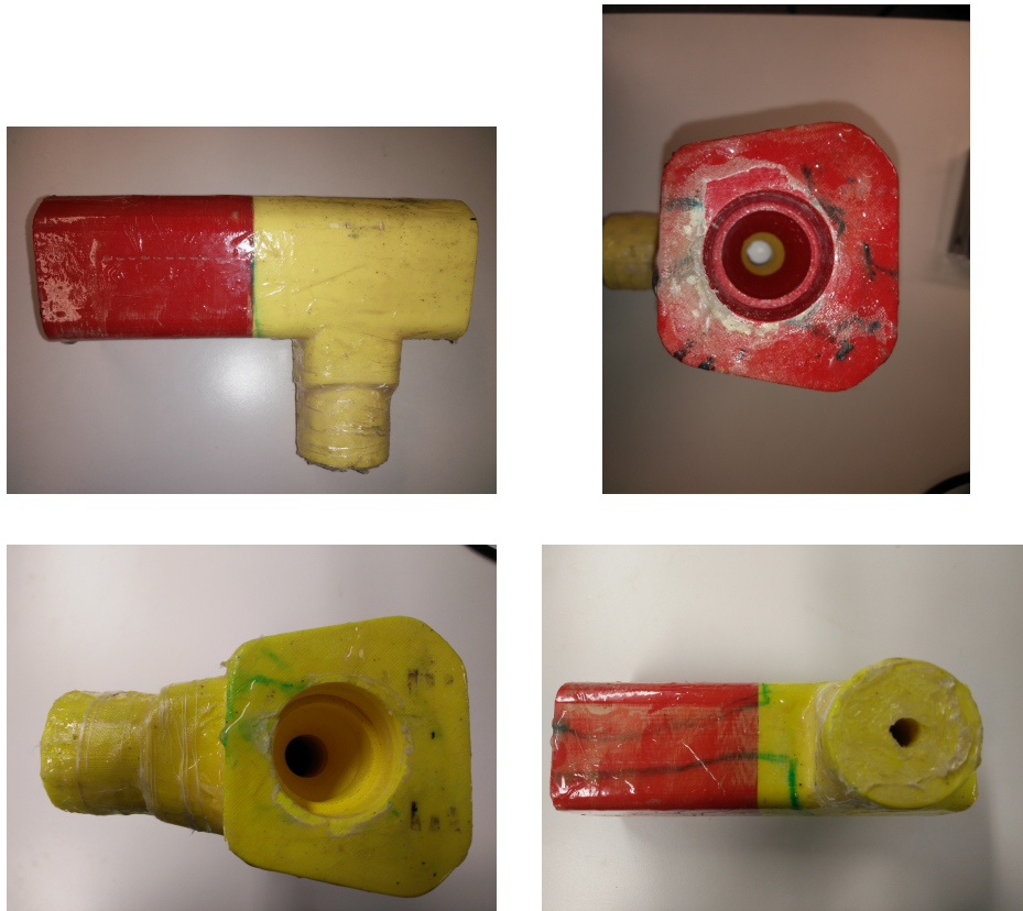
Figure 5.1: 3D printed plastic venturi for particle injection
