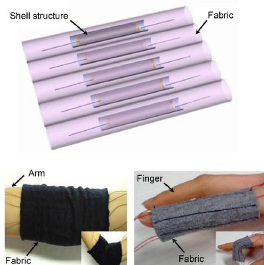
Figure 8 - Piezoelectric fabric with incorporated shell structure [28] .
