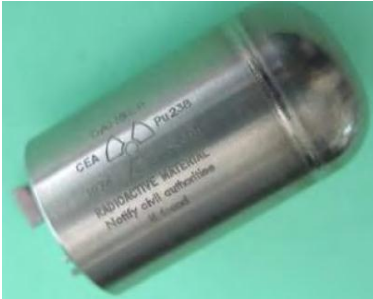
Figure 4 – the Laurens-Alcatel battery for Medtronic devices used Plutonium 238 and converted thermal energy using a thermopile [16] .
