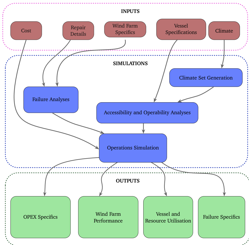
Figure 1.2: A schematic diagram depicting the Strath OW O&M tool and its basic principles of operation.
