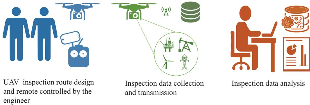
Figure 1.1: Scheme of UAV-based visual inspection
