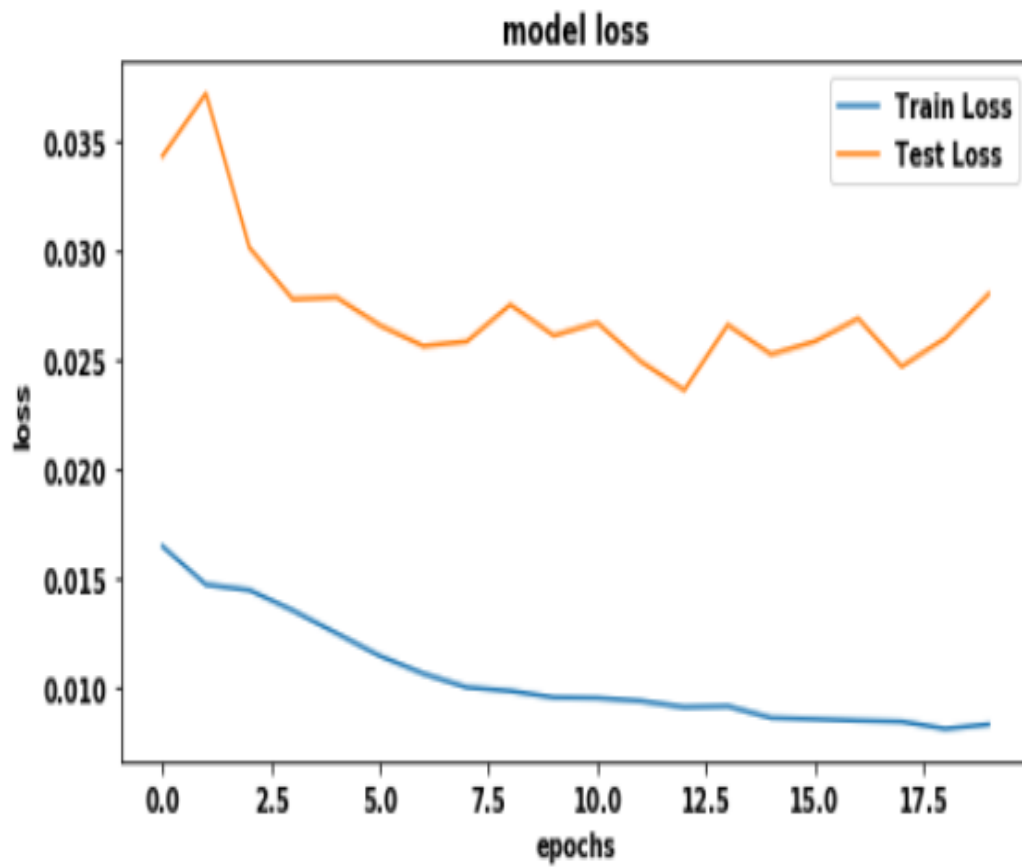
Fig. 5.26. 24 time step Loss plot for multivariate CO_2 prediction with LSTM model using Post-Doc dataset
