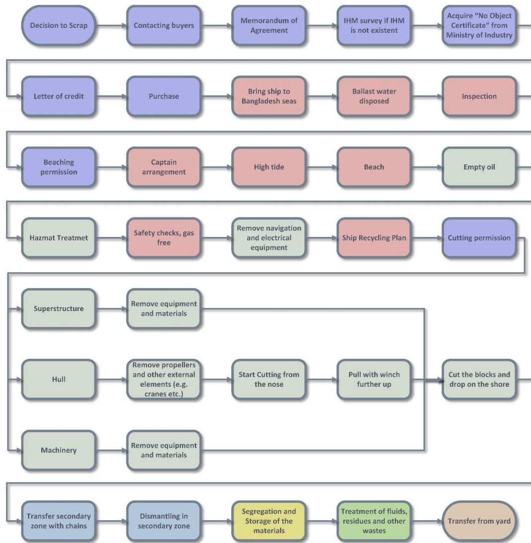
Figure 4.12: Step by step ship recycling process in Bangladesh
