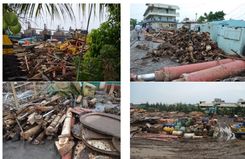
Figure 4.16: Segregation and store zones in a Bangladeshi Ship Recycling Yard (Chittagong – Bangladesh. October 2015)
