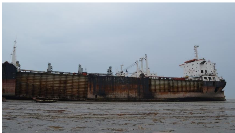
Figure 4.14: Ship in the primary cutting zone, propellers and side plates of the ship are removed (Chittagong – Bangladesh. October 2015)
