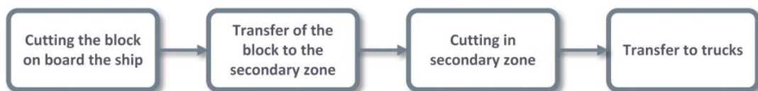
Figure 7.11: Dismantling process for the data collection study
