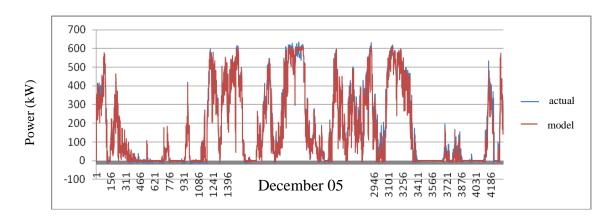
Figure 5.18a: Power model output for a healthy turbine (T15) during December 05.
