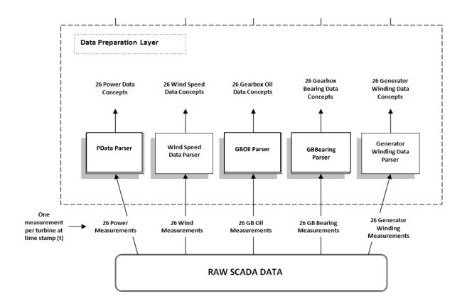
Figure 6.5: Summary of Data Flow through Data parser Agents (the data preparation stage)
