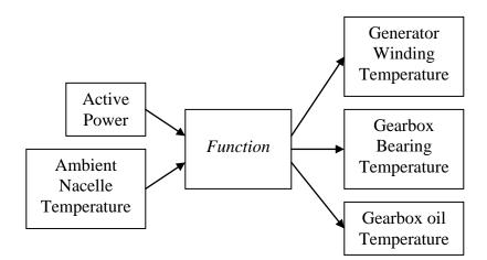
Figure 3.1: SCADA Data parameters relations
