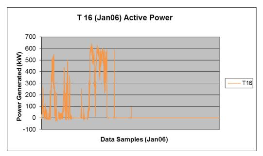
Figure 5.4a: Active power falls to zero once fault occurs
