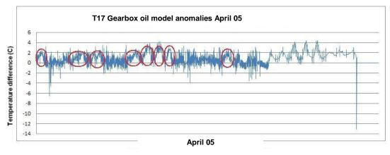
Figure 5.16b: Gearbox problems: cooling oil model error signal anomalies detected in T17 April 05.
