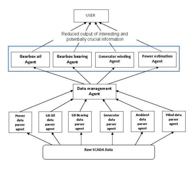
Figure 6.1: The Proposed System Architecture
