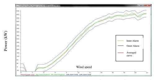
Figure 5.19a: Learned curve for T8 from healthy period of operation before generator failure
