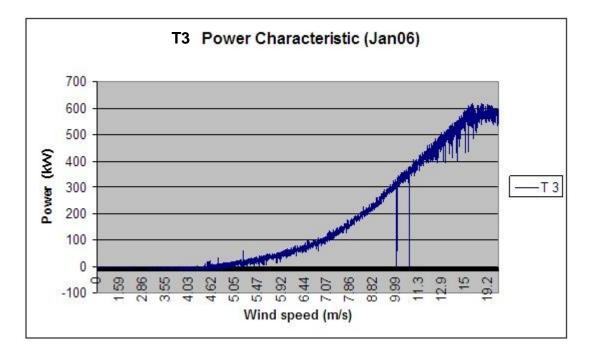
Figure 5.3: T3's Power Characteristic for the month of January 06 (Data is sorted in ascending order for the month)
