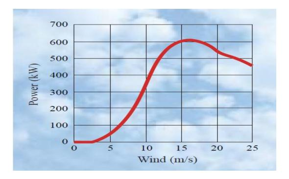
Figure 5.2: Bonus 600kW Manufacturers Power Curve
