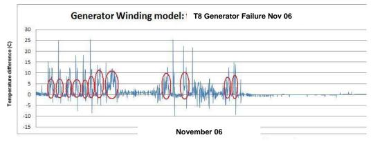
Figure 5.17b: Generator Failure: corresponding error signal
