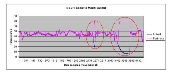
Figure 5.12: 4-5-3-1 Gearbox oil Specific Model showing signs of over-fitting when tested against the data for the month of November 06
