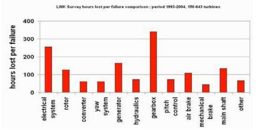
Figure 2.4: Downtime hours associated with various turbine components (Tavner et al 2006)
