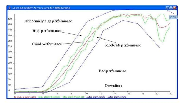
Figure 5.20: Power and wind data pairs are classified into the shown groups according to which alarm limits they fall within.
