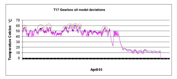
Figure 5.16a: Gearbox problems: detected by gearbox cooling oil model in T17 April 05.
