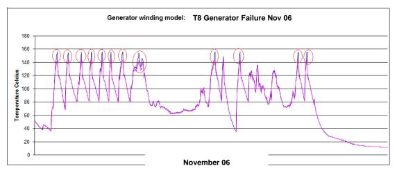
Figure 5.17a: Generator Failure or brought offline (November 06) detected in Generator Winding temperature parameter.
