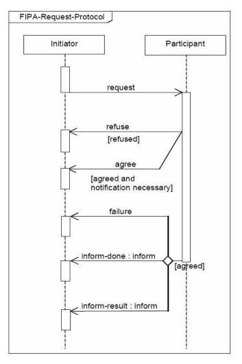
Figure 4.5: The FIPA Request Interaction Protocol (FIPA 2002c)
