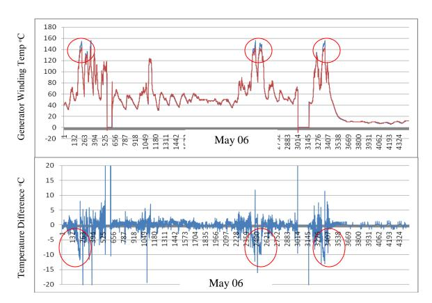
(shown in Appendix I) in the months of June and September before the generator finally fails in Novmeber 06.
