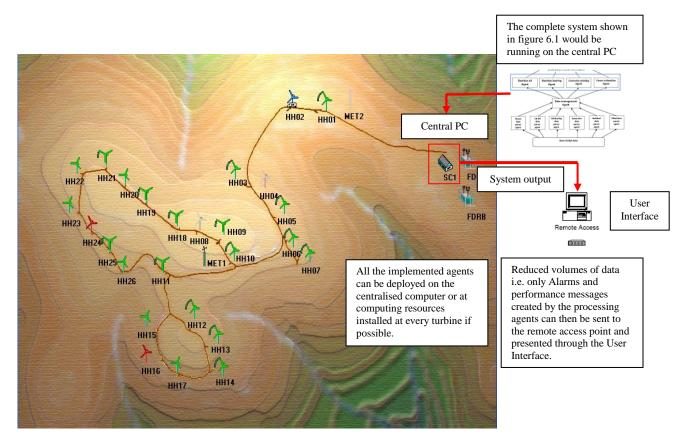
Figure 6.9: SCADA Wind farm network infrastructure
