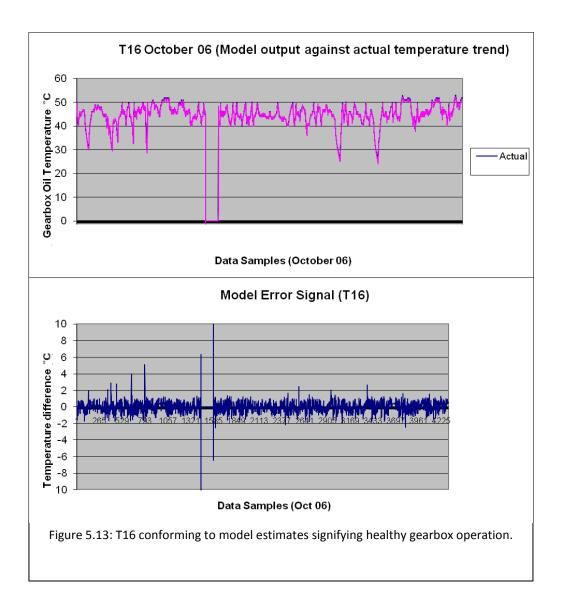
As can be seen from the error signal obtained the majority of the differences lie between the ranges of -2 to  $2^{\circ}$ C. There is no consistent positive or negative divergence between the two signals for a sustained period of time.
