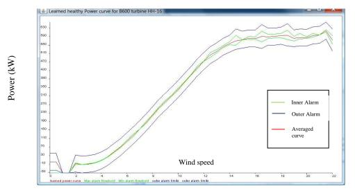
Figure 5.19c: Learned curve for T16 from healthy period of operation before gearbox failure.
