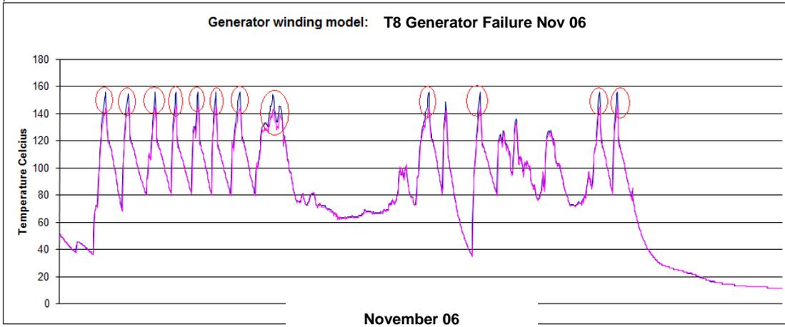
Figure 5.17a: Generator Failure or brought offline (November 06) detected in Generator Winding temperature parameter.
