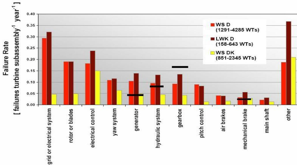
**Figure 2.3: Distribution of failure rates of wind turbine components from 3 surveys (WSD, WSDK, and LWKD) averaged over 11 years from over more than 7000 turbines. (Tavner et al 2006)**
