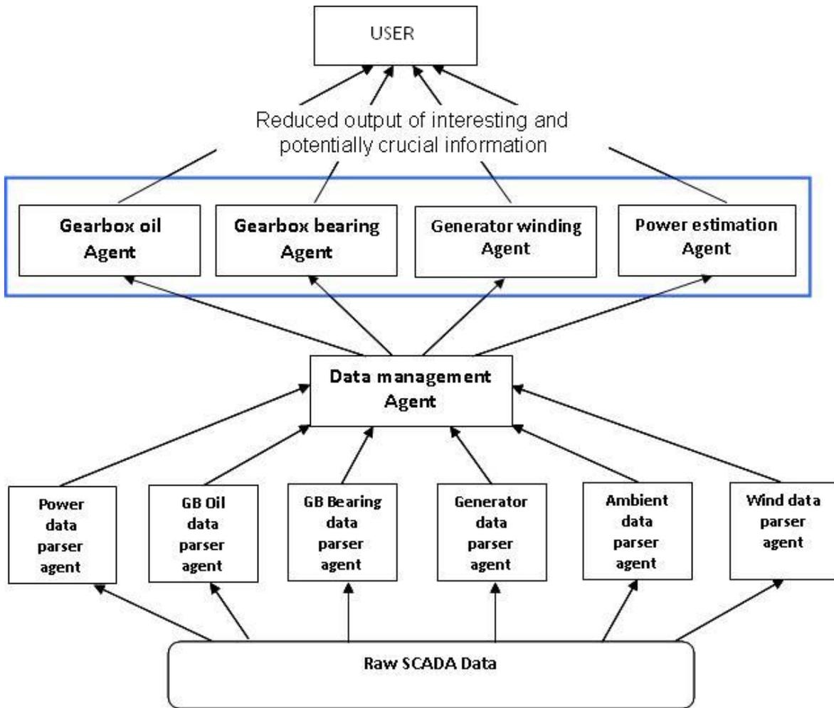
**Figure 6.1: The Proposed System Architecture**
