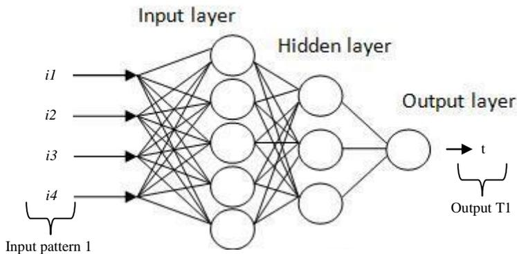
**Figure 3.5: Back Propagation Neural Network Architecture**
