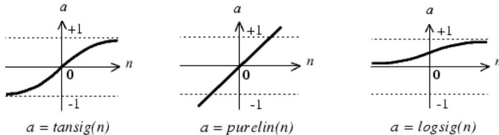
**Figure 5.9: The different neuron transfer functions available in the MATLAB toolbox (MATLAB NN 1984-2007)**
