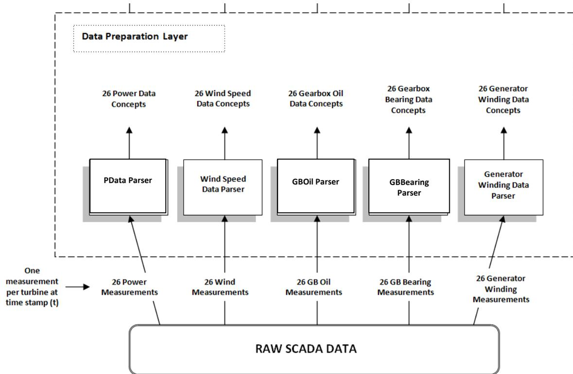
Figure 6.5: Summary of Data Flow through Data parser Agents (the data preparation stage)
