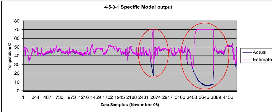
**Figure 5.12: 4-5-3-1 Gearbox oil Specific Model showing signs of over-fitting when tested against the data for the month of November 06**
