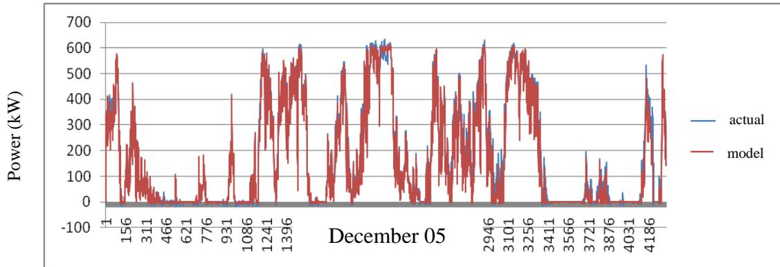
**Figure 5.18a: Power model output for a healthy turbine (T15) during December 05.**
