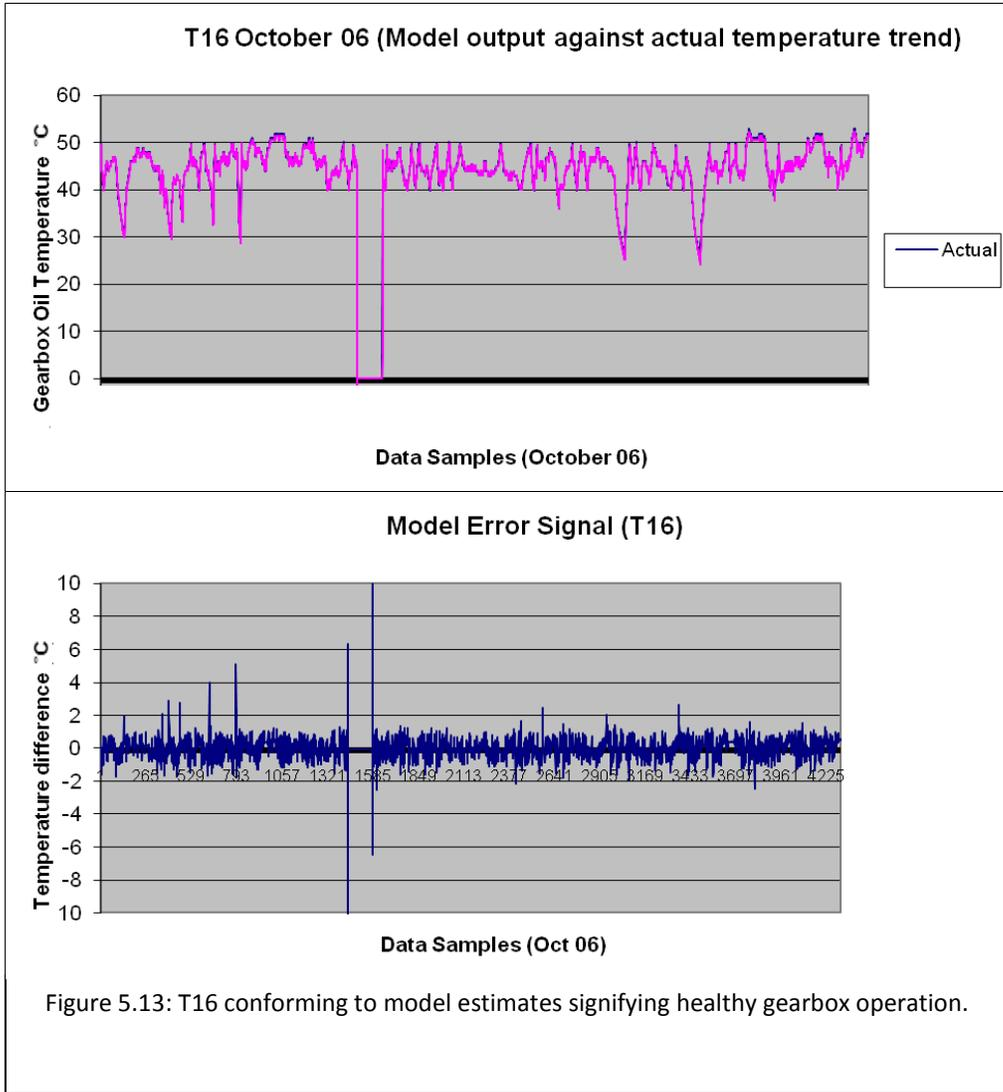
As can be seen from the error signal obtained the majority of the differences lie between the ranges of -2 to 2°C. There is no consistent positive or negative divergence between the two signals for a sustained period of time.
