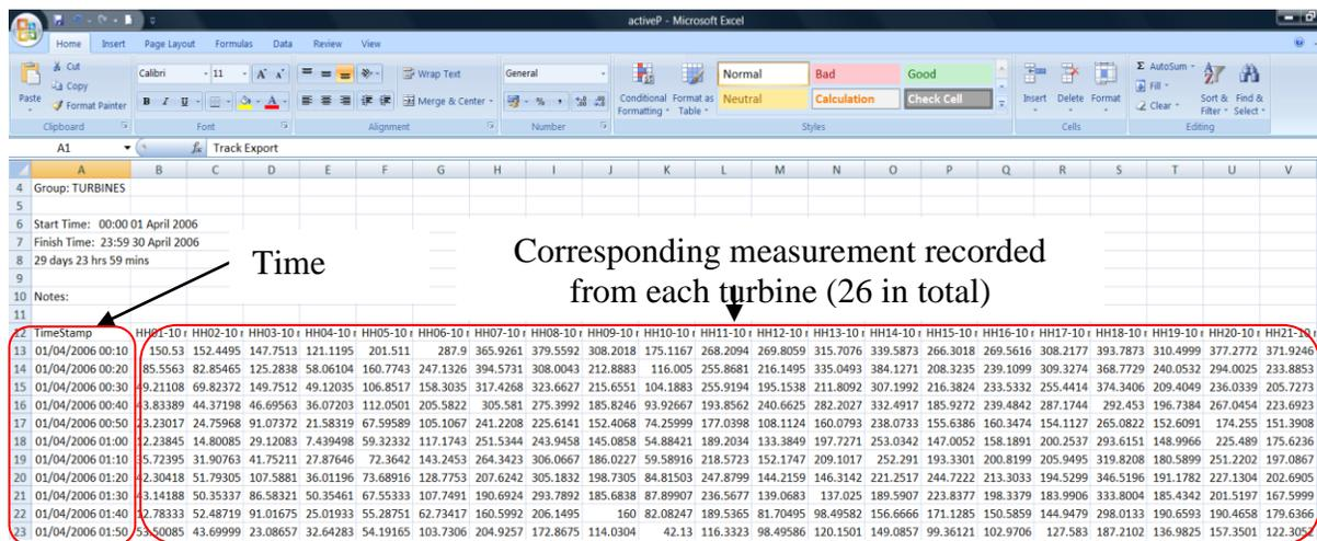
Figure 6.4: Extract from Exported SCADA file from SCADA Database
