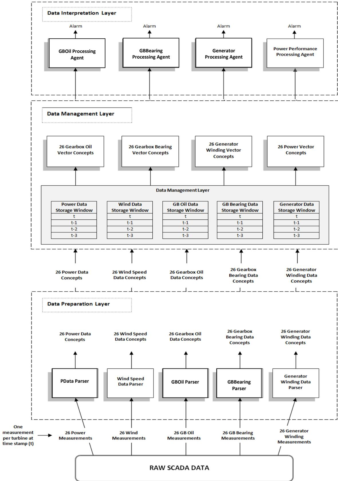
Figure 6.8: The Data Flow through the System's Various Layers
