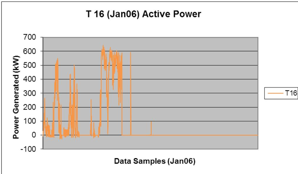
Figure 5.4a: Active power falls to zero once fault occurs
