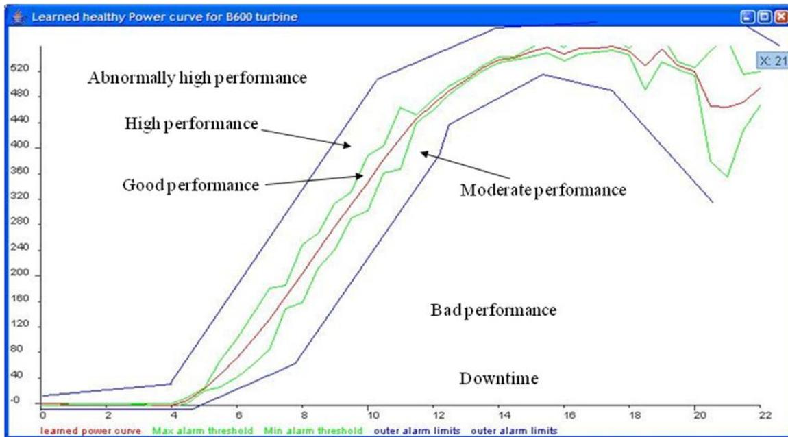
**Figure 5.20: Power and wind data pairs are classified into the shown groups according to which alarm limits they fall within.**
