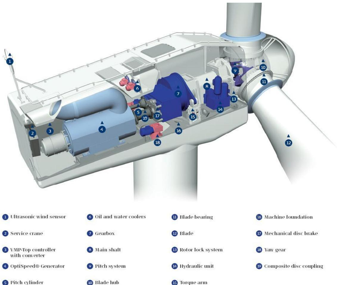
Figure 2.2: the internals of a Vestas V52-850kW turbine (Vestas 2009)
