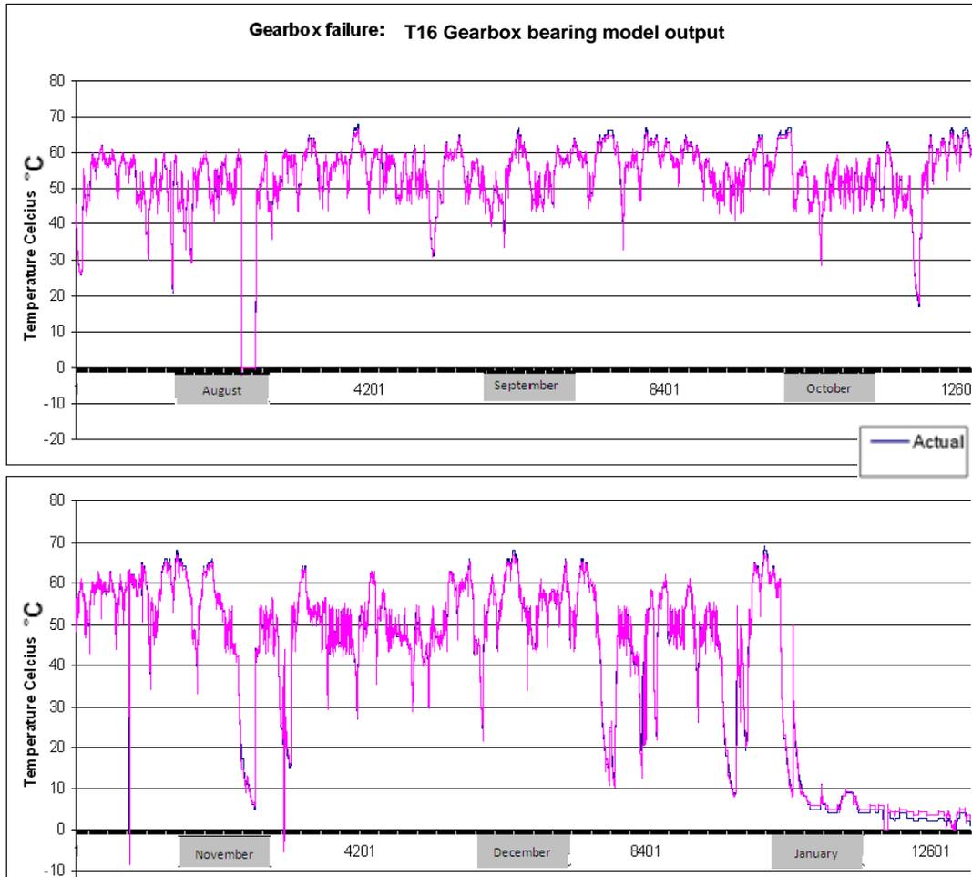
**Figure 5.15a: Gearbox failure detected: Corresponding gearbox bearing model output detected during aug05-jan06.**
