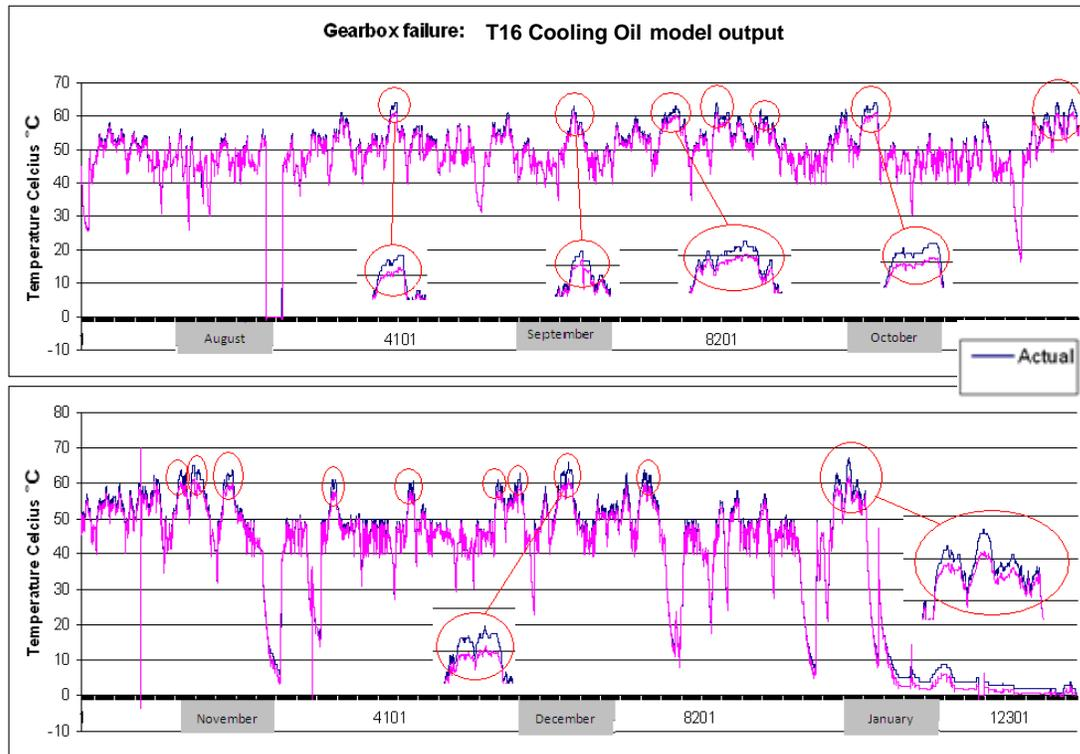
**Figure 5.14a: Gearbox failure detected T16: gearbox cooling oil model output, anomalies detected from aug05-jan06.**
