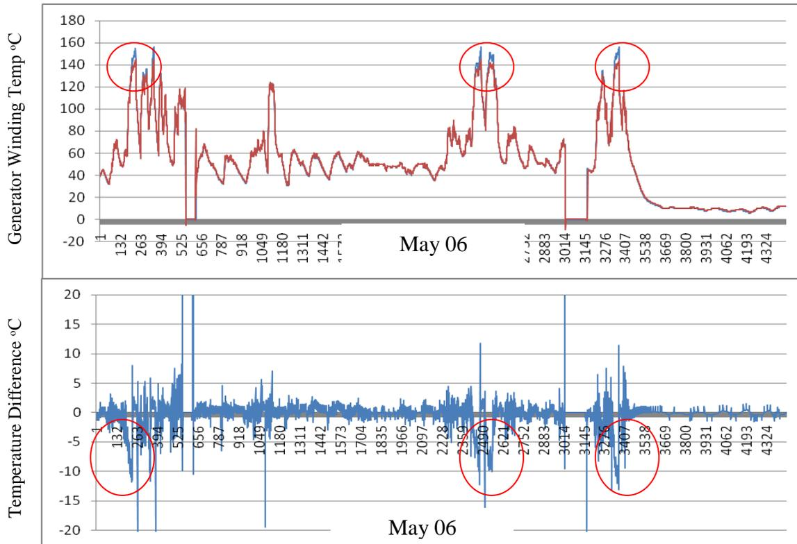
**Figure 5.21: Generator Temperature anomalies for T8 during the month of May06.**
