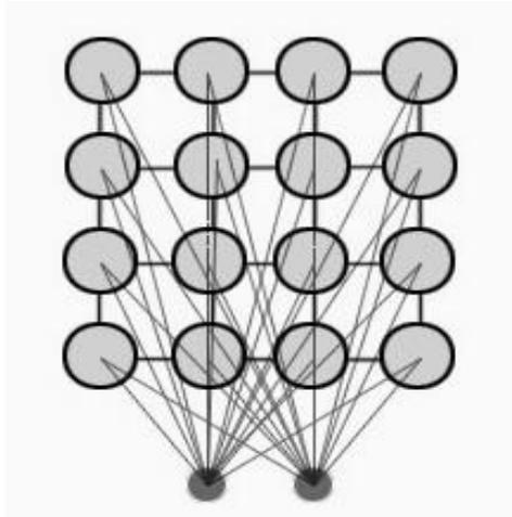
**Figure 3.2: A 4 x 4 Node SOM with a 2 input vector**
