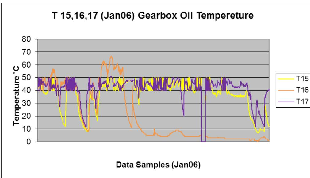
Figure 5.4b: gearbox oil temperature of T16 compared to neighbouring turbines
