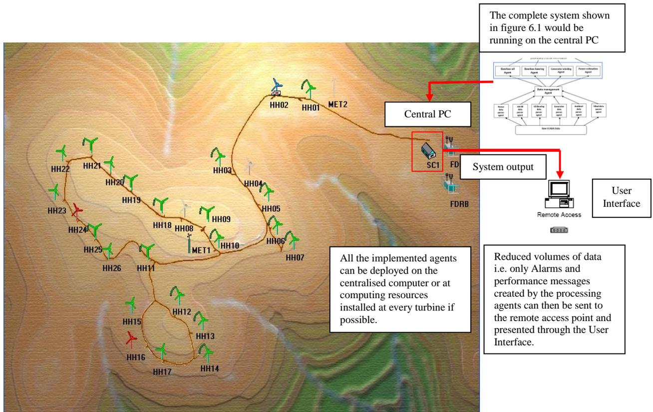
Figure 6.9: SCADA Wind farm network infrastructure
