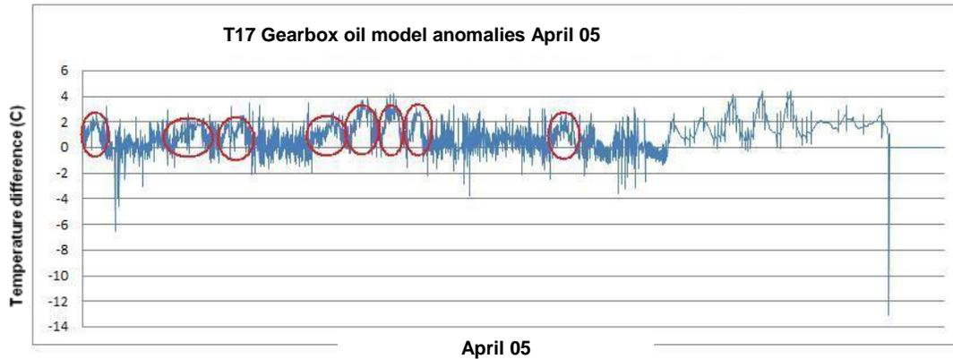
**Figure 5.16b: Gearbox problems: cooling oil model error signal anomalies detected in T17 April 05.**
