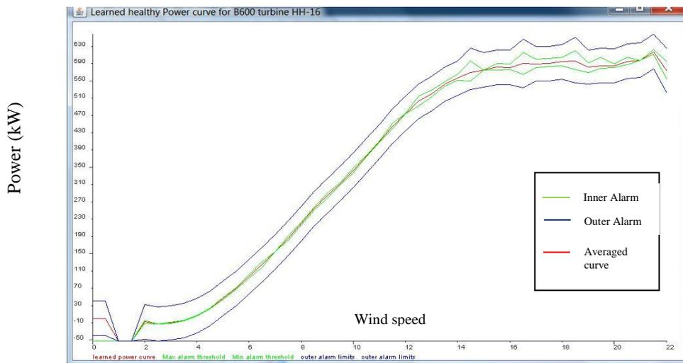
Figure 5.19c: Learned curve for T16 from healthy period of operation before gearbox failure.
