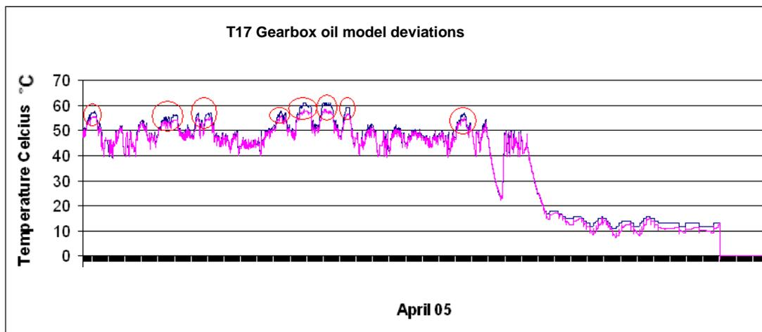
**Figure 5.16a: Gearbox problems: detected by gearbox cooling oil model in T17 April 05.**
