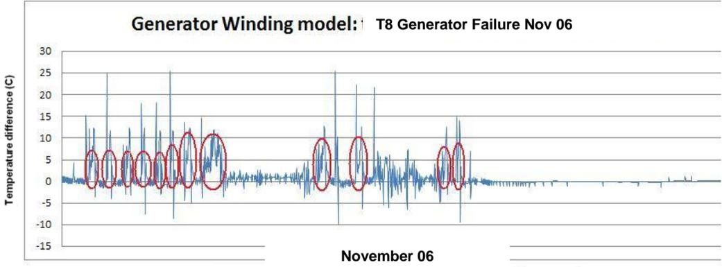
Figure 5.17b: Generator Failure: corresponding error signal
