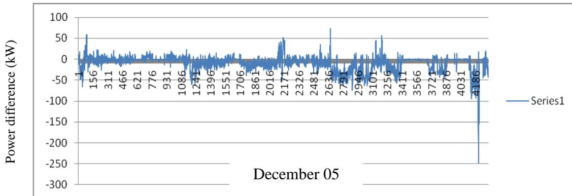
**Figure 5.18b: The corresponding error signal between actual data and the model estimation during December 05.**
