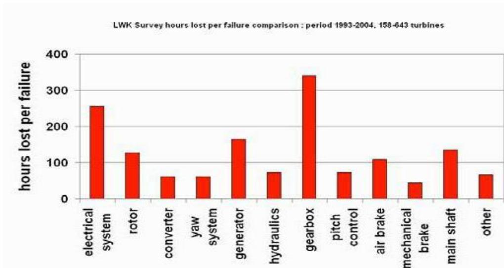
Figure 2.4: Downtime hours associated with various turbine components (Tavner et al 2006)
