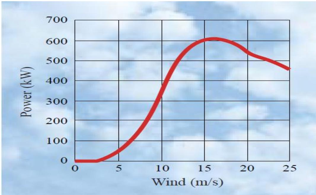
Figure 5.2: Bonus 600kW Manufacturers Power Curve
