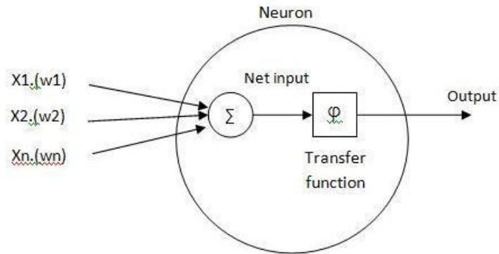
**Figure 3.4: The Perceptron processing element**
