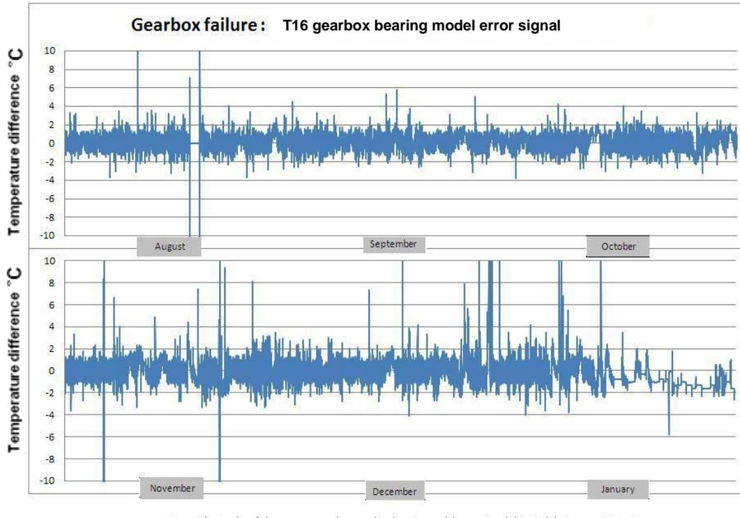
**Figure 5.15b: Gearbox failure detected T16: gearbox bearing model error signal detected during aug05-jan06 showing no significant or prolonged periods of deviation.**
