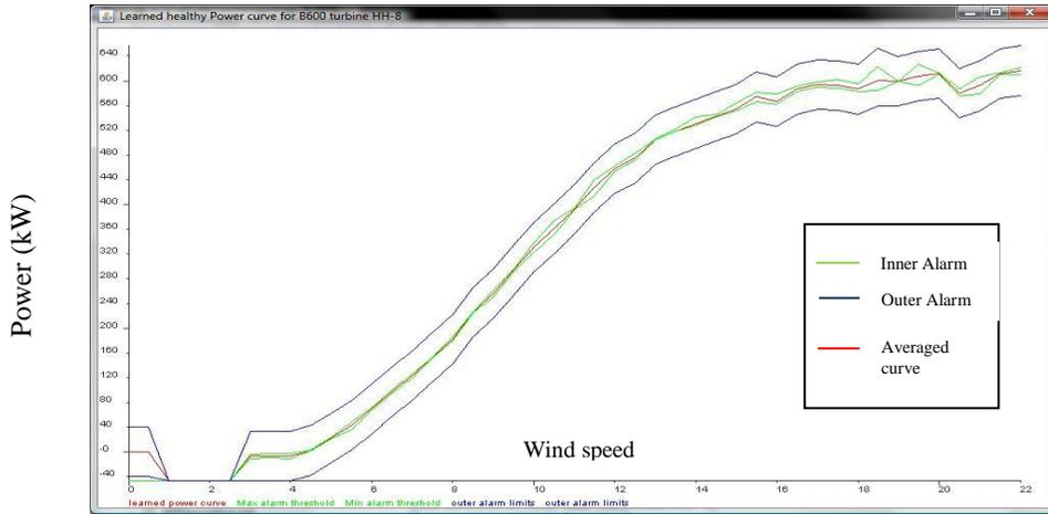
Figure 5.19a: Learned curve for T8 from healthy period of operation before generator failure
