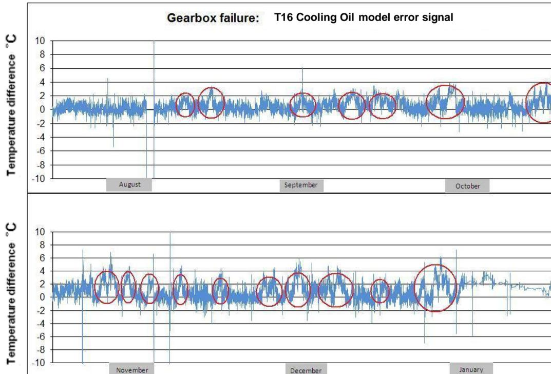
**Figure 5.14b: Gearbox failure detected: gearbox cooling oil model error signal, anomalies detected from aug05-jan06.**
