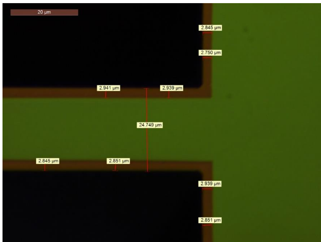
Figure 3.10. Microscope image of SIRE grooves after KOH etch. Blacked out areas are deep grooves and everything else is a Nitride hard mask. Due to thin film reflection effects, light scattered from Nitride lying atop silicon appears green, and Nitride suspended in air appears brown [31]. Measuring the overhanging Nitride indicates the grooves are ca. 6 \mu\text{m} wider and longer than intended. Images acquired using a reflectance spectrometer.
