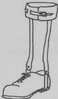
Figure 3.1: Conventional metal and leather AFO with double uprights (McHugh, 1987).
