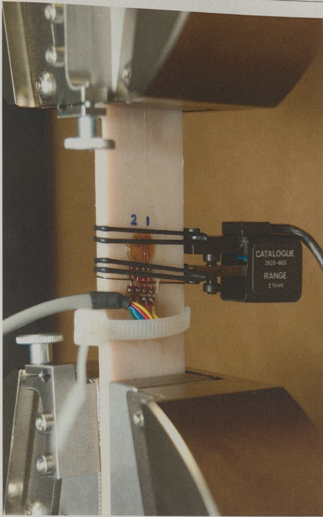
Figure 4.3: Particulars of the sample showing strain gauge and extensometer.
