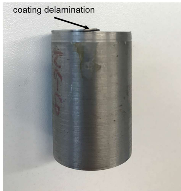
Fig. 2-13 Photograph illustrating the coating delamination on WC-CoCr test specimen 2
