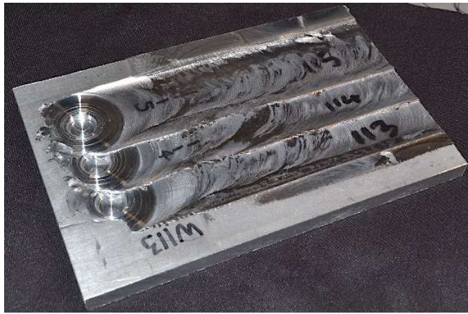
Fig. 7-21 Macroscopic image showing the surface of the SprayStirred \text{Cr}_3\text{C}_2\text{-NiCr} specimen with 10 mm overlap
