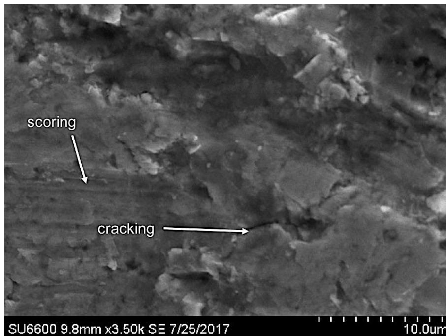
Fig. 5-20 SEM micrograph of the worn surface on the \text{Cr}_3\text{C}_2\text{-NiCr} coated specimen following slurry erosion test at 90^\circ impingement [x3500]
