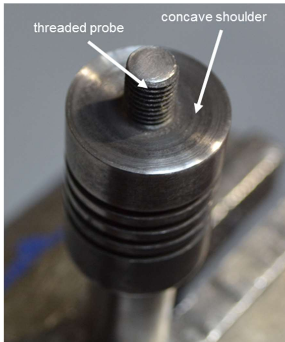
Fig. 2-3 FSP tool with concave shoulder and threaded probe
