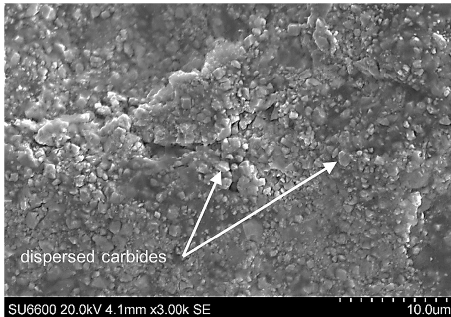
Fig. 7-34 SEM micrograph of the impinged SprayStirred WC-CoCr reinforced MMC [x3000]
