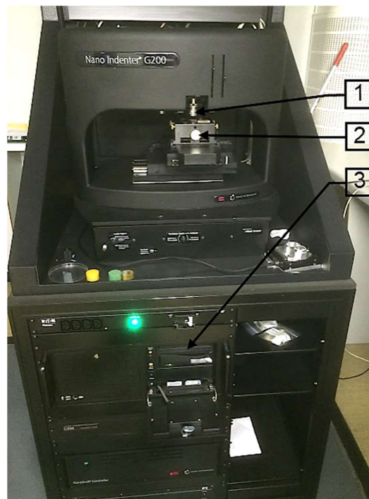
Fig. 4-7 Agilent Nano Indenter G200; (1) Berkovich indenter, (2) specimen stage, (3) data logging
