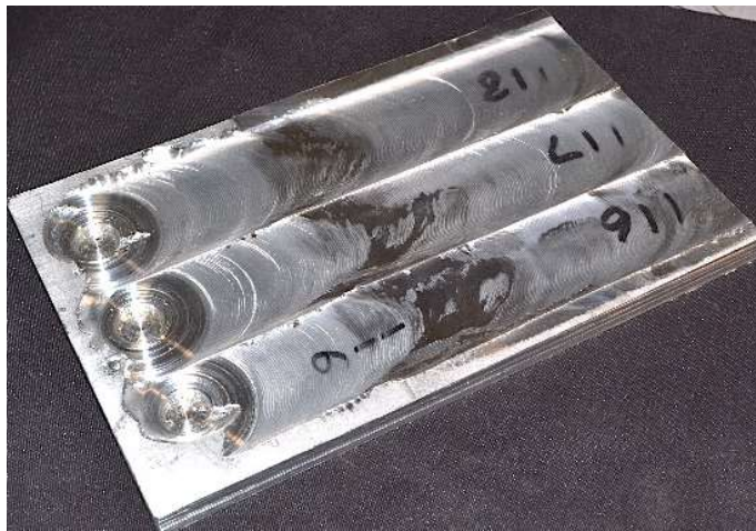
Fig. 7-22 Macroscopic image showing the surface of the SprayStirred \text{Cr}_3\text{C}_2\text{-NiCr} specimen with 5 mm overlap
