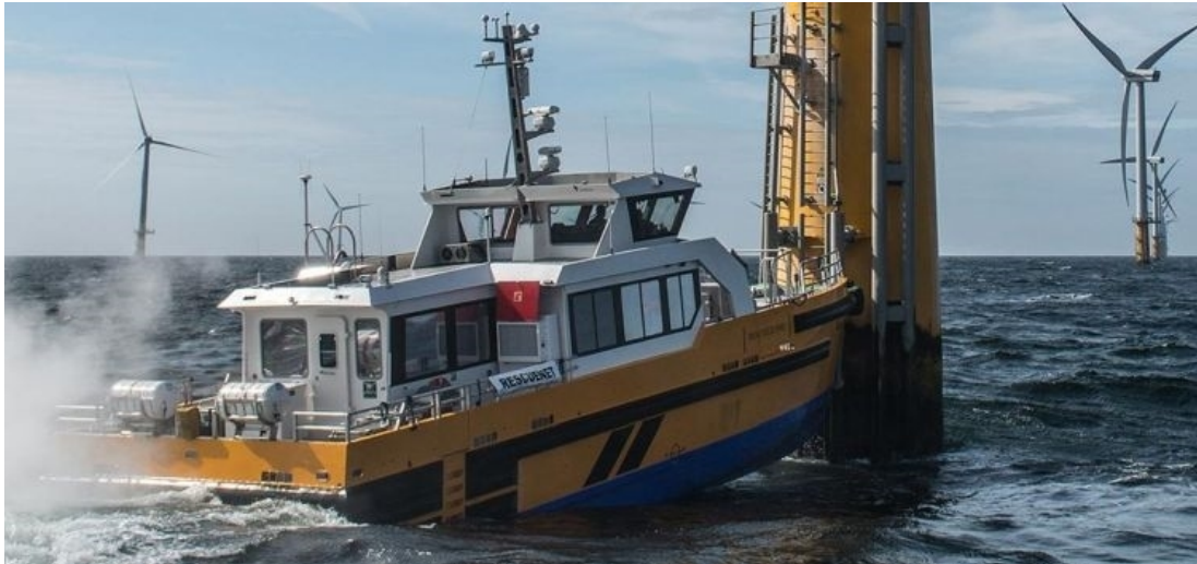
Figure 2.3. CTVs remain in place during crew transfers by pushing on against the transition piece 5 .
