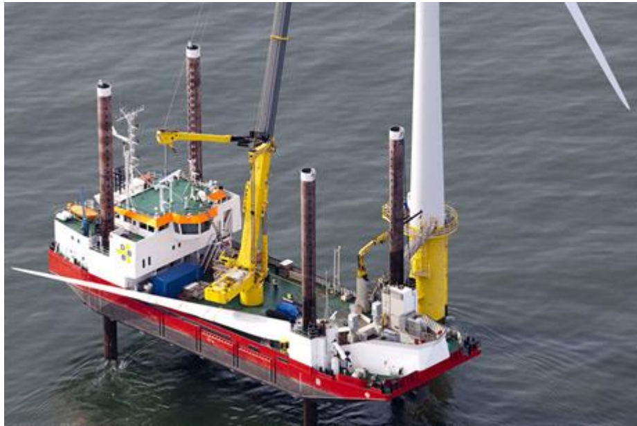
Figure 2.5. Jack-up vessels used for major component replacements 6 .
