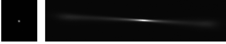
Figure 4.3: Example of beam distortion from a diverging scanline at the target plane, from an early version of the addressing setup. The beam has a waist of 38\ \mu\text{m} with the MEMS scanner at rest (left). Scanning produces a 1.89\ \text{mm} wide scanline, but deforms the beam to a waist of approximately 175\ \mu\text{m} at the edges of the scanline (right). These images were obtained using a Thorlabs DCC1545M CMOS camera
