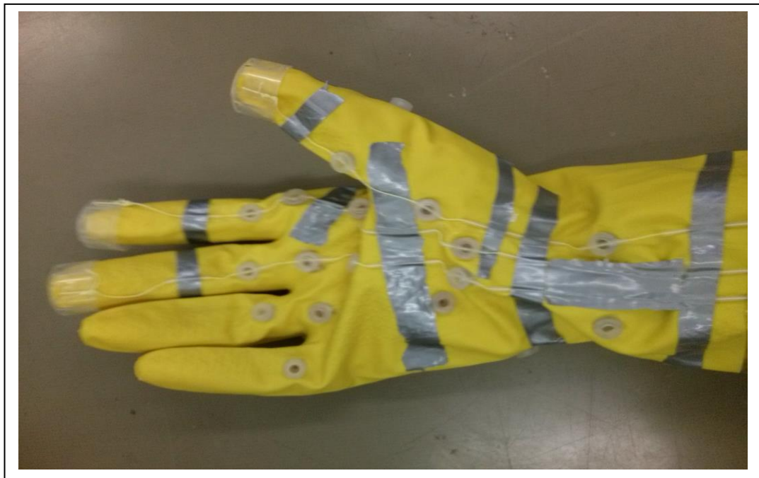
Figure 12: Photograph of an early model inner layer for the prototype displaying the cable pathways. The final model inner layer had the tape removed as it restricted movement [231].
