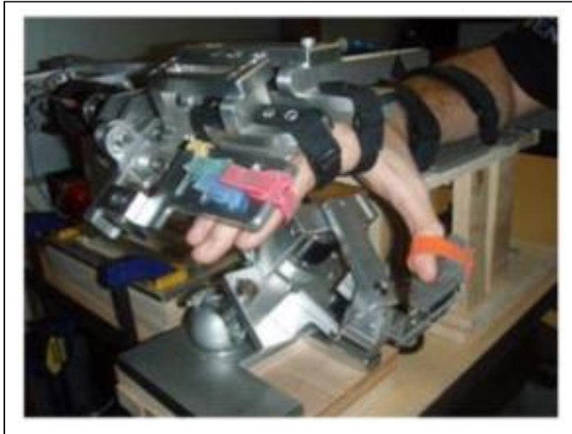
Figure 1: Image of the HEXORR Device with the Wearer's Hand in Extension and the Thumb in Full Abduction [101].
